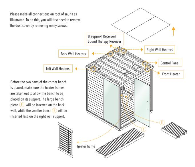
The floor heaters **G** will need to be connected to the right wall wires. The diagram to the right shows where the connection is made. You will need to remove the floor grate and a small hatch covering the harness.
