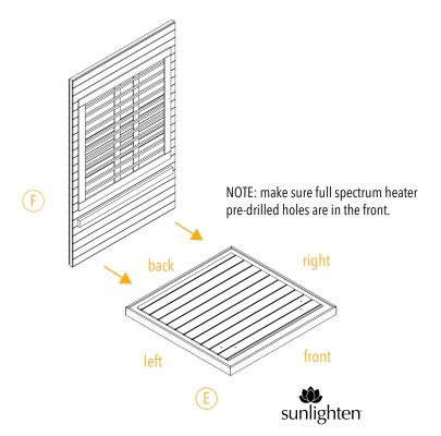
Place right wall **G** on the right side of floor panel **E**. This wall panel should sit flush once properly seated. Make sure no gaps are visible in the corner of the two walls as you insert it. It should be inserted flush.
