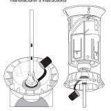
Return shroud to upright position after finishing operation. Leave tubing attached to tube-fed safety syringe and quick-fit connector until dosing equipment has been removed from the shroud. Remove dosing equipment by pushing the trigger as shown in the picture, then disconnecting the quick-fit connector from the
