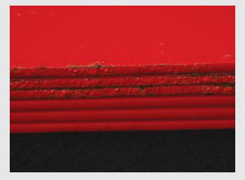
This image of laser-cut edges highlights the edge corrosion performance of a standard DTM powder coating (top 3 panels) versus PPG's High Edge DTM powder (bottom 3 panels) after 40 cycles of cyclic corrosion testing as per SAE J2334.
