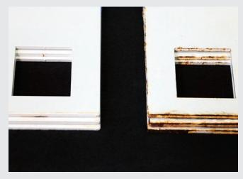
This image of laser-cut edges highlights the edge corrosion performance of a standard DTM powder coating (3 panels on the right) versus PPG's High Edge powder (3 panels on the left) after 40 cycles of cyclic corrosion testing as per SAE J2334.
