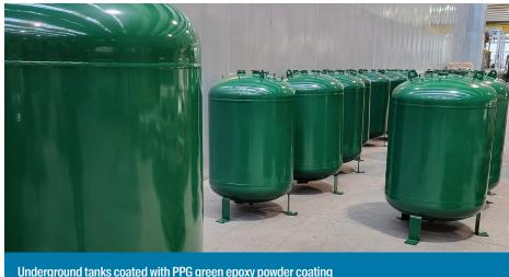
Underground tanks coated with PPG green epoxy powder coating at Antonio Merloni Pressure Vessels' plant in Matelica
