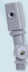
Photocell Stem and swivel type. 120V, 6A, 1 650W to 277VAC, for HID or LED fixtures. # INTEK4236S
