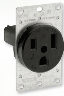
Flush mount 50A, 2P, 3W, NEMA 6-50R # LEV5374S00
