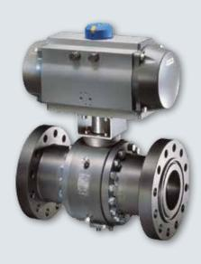
**SAMSON** VETEC – VETEC's Maxifluss valves combine the advantages of conventional control valves, butterfly valves and ball valves. Their universal design allows them to be used in standard and critical applications. Thanks to the eccentric design of the rotary plug, it only comes into contact with the valve seat when the valve is completely closed. This means that the valves can control at high rangeability.
