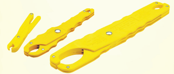
Medium Fuse Puller 250V 5 in - 9/32 to 1/2 in diameter # IDE34001 0-100A, 250V and 600V 7-1/2 in - 1/2-1 in diameter # IDE34002 0-100A, 250V and 600V 11-3/4 in - 1/2-1 in diameter # IDE34003
