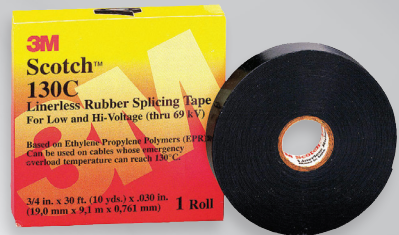
Linerless Rubber Splicing Tape 3/4 in x 30 ft - 30 mil. 130C, black. # TRO130C3/4X30
