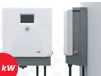
Terra DC Wall Charger Level 3 charging station Fast and compact 24 kW direct current charger including RFID reader, Ethernet connection and CCS1 sockets. Other configurations available. Contact your Lumen representative for more information. Single phase # ABBTERRA1PH24KWCCS1 3-phase # ABBTERRA3PH24KWHCCS1
