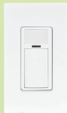
Smart Sensor 120 / 277VAC, 50 / 60Hz, PIR, antimicrobial, app configurable: manual ON / Auto-OFF selectable, neutral wire required, white. Wallplate not included. # LEVODS15IDW
