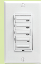
Electronic Timer Switch 120VAC, 60 Hz, 1 800W incandescent, 20A resistive / inductive, 1HP, single pole, 3-way. Wallplate not included. 5-10-15-30 minutes # LEVLTB301LZ 10-20-30-60 minutes # LEVLTB601LZ
