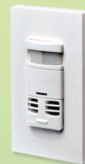
Multi-Tech Occupancy Decora Sensor 120 / 277V, 50 / 60Hz, single pole, 60° or 180° field of view, 2 400 ft 2 coverage, 10 to 30 minute time delay. Wallplate not included. # LEVOSSMTMDW
