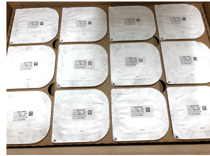
Packaging used for interplant shipment of Surgical Structural Heart implant devices was redesigned from a 24-pack to a 48-pack style. The new design reduces packaging materials by 31.8%. Anticipated packaging waste reduction from the new design will be 1,241 kg per year.
