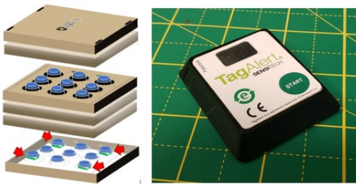
Heart valve packaging previously required 36 TagAlerts® per box. Newly redesigned packaging allows for just 4 TagAlerts® per box, resulting in an 88% packaging weight reduction and anticipated packaging waste reduction of 2,766 kg per year. TagAlerts® must be disposed as electronic or hazardous waste in many countries; therefore, this project reduces both overall packaging waste and customer regulated waste.
