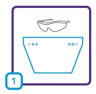
Unpack Face Shield from box and locate a pair of safety glasses to attach to the Face Shield.
