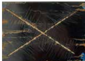
Conventional Ecoat CRS - 15' @ 175°C (347°F)
