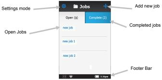
**Add New Job:** This mode is the main mode of operation. Sample measurements are taken, saved and analyzed in this mode.
