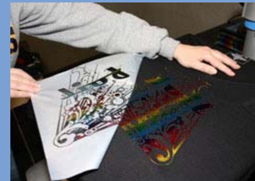
4. Peel foil, only adheres where ink transfer had been applied
