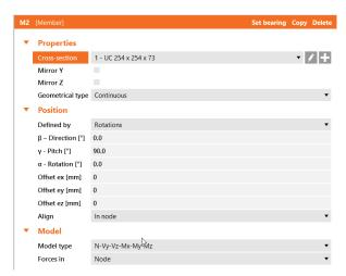
Notice that this time we have to change the cross-section using the plus symbol. If we edit this section to a PFC then both the column and the new beam will be that shape. This is because IDEA StatiCa uses a connection library of members that we add to, copy and edit.
