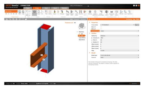
Member 2 now must be aligned to the outer face of the column. The view that we are currently in isn't very conducive so we need to change our viewpoint. We can either hold down the Ctrl key and the middle mouse button or use the view cube to 'spin' the view so that we are able to see both faces of the column and beam that we want to align or we can simply pick another corner of the view cube. This aligns the view to one of several pre-defined viewpoints. You can do the same with any edge or
