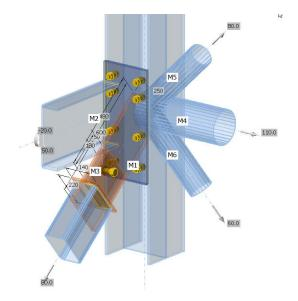
The tongue of the connection needs adjusting to make it more visually appealing. Built-in to the connection is a plate editor. Within the orange band where the properties of the operation are described you will find the editor with a drop-down arrow. If you expand this you will see several entries. The one we are going to edit is the tongue.
