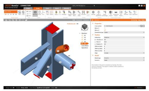
To place the final member we are going to copy M5 and adjust its orientation as most of what we need is already defined.
