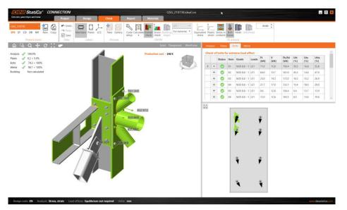
Here we can see the bolt forces in the workspace and the calculations related to each bolt in the righthand panel. The resultant forces are shown pictorially as well.
