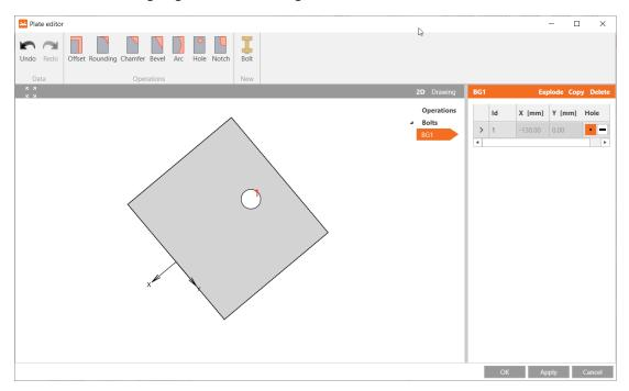
Currently we see a rectangular plate. We would like to take off a 30x100 bevel from each of the corners nearest the hole. When you select bevel the plate editor shows an example bevel on corner 1. The editor has annotated the corner numbers (the nearest number to the corner). The two corners we want to amend are 1 and 2. As you change the values the appearance of the plate changes in the editor. Pressing Apply will commit these changes to the plate and pressing OK to the model.
