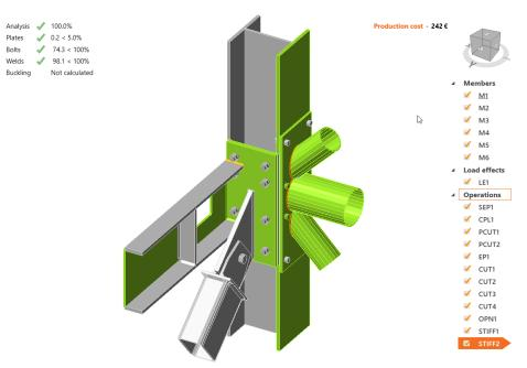
What does this mean? The calculate option from the Design tab of IDEA StatiCa Connection presents the results in a traffic light format. Grey is under-utilised. Green is ok. Amber is up to 100% and red is over 100%. Needless to say, red is where you have problems! There is also a useful summary in the top right-hand corner of the workspace. In this example we have no red indicators (which is good),
