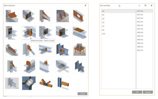
You are required to nominate a grade and size of bolt for this connection first. We shall try M20/8.8 bolts. Select OK to continue.
