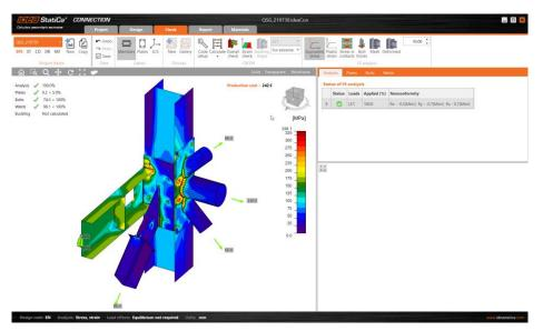
We can also investigate items in isolation by changing the focus of the right panel in the orange bar to say Plates. Here we can look at each plate and the stresses etc in turn.
