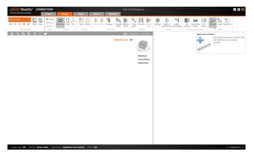
To add the column (M1) we go to Add a new member from the toolbar (or you can also right mouse click on Member in the Workspace and select New member). This brings up the following dialog which allows you to choose a suitable cross-section. As you can see there are many different types of cross-section but we are concerned with Rolled I section (top left).
