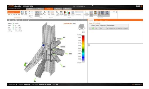
We can use this option to get feedback to see if the joint is behaving generally as expected. The additional checks might direct us to examine the strains around holes in plates for instance or we might want to control the stresses in the webs of members. All is possible to arrive at a sensible overall joint design. There are many tutorials on our web site that will take you through many different types of analysis and verifications.
