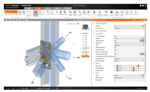
The new gusset plate is not related to anything so select the X. This has an immediate effect on the plate that was connecting to member M1 in that it now aligns to the brace axis. Make sure that X is selected in the also related to field as we want this plate to be considered in isolation.
