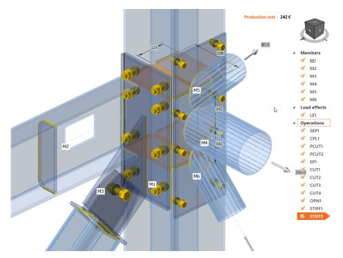
The connection is now complete and the next step is to perform an analysis. Notice that some operations are not in the same order as you would fabricate this item. Hopefully, you can see why this is the case and have gleaned an initial understanding of how a connection goes together.
