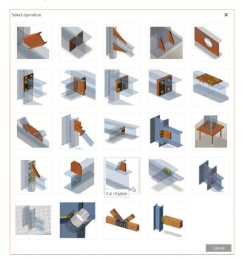
We are going to modify the gusset plate. Use the plate option and arrow to select the correct plate. It is going to be cut by the existing flange plate. Again, set the plate option and arrow to select the correct plate. You can experiment with the + and – options for remaining part and surfaces.
