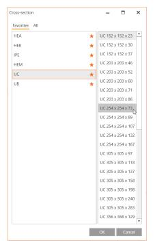
When you picked the correct section and then select OK this is inserted back into the previous input screen and now we can allocate the correct steel grade. You will see both a pencil and a plus symbol. The pencil allows you to edit what is currently indicated. However, it is not a good idea to edit a standard grade of steel unless you really need to!
