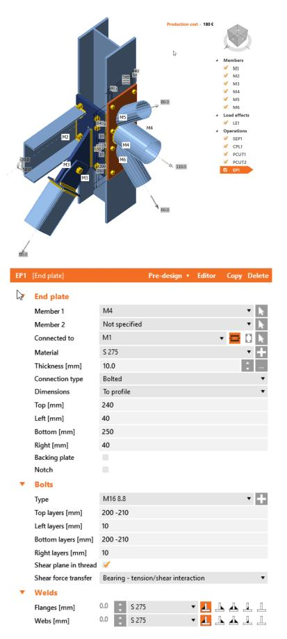
We now need to cut and cope members M5 and M6 using the cut operation four times.
