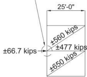
Typical bracing elevation
