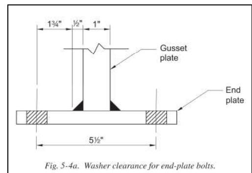
Fig. 5-4a. Washer clearance for end-plate bolts.
