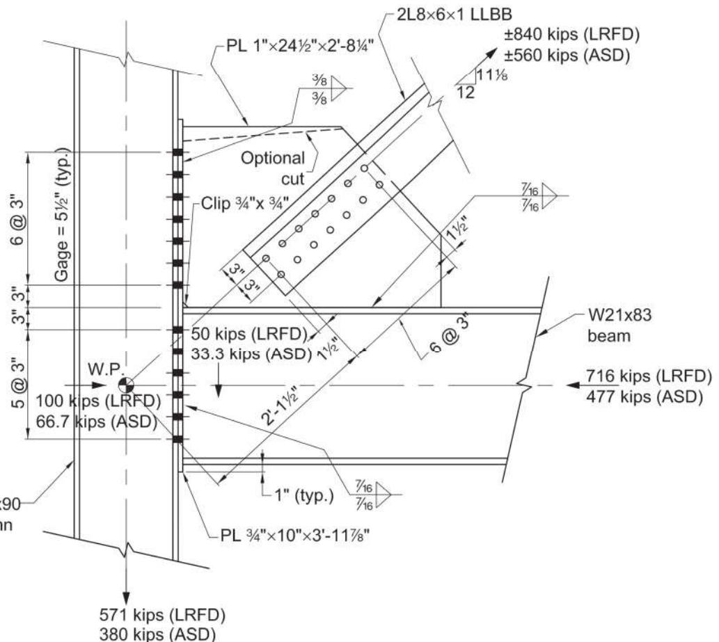
Fig. 5-1. Strong axis bracing connection—general uniform force method.
