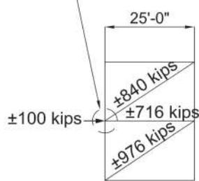
Typical bracing elevation
