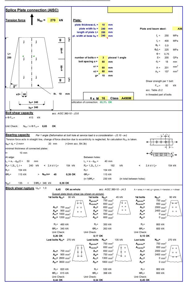
The resulting shear force in one bolt is:  $\mathbf{Fnv} = \mathbf{N} / 6 \text{ bolts} = 270/6 = 45 \mathbf{kN}$
