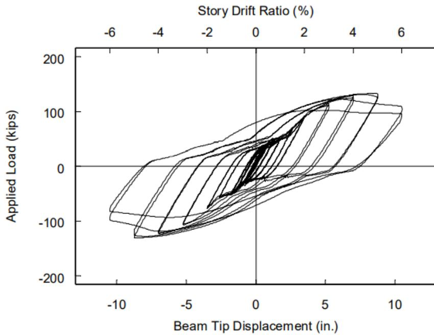
Figure 3.6: Moment at column face-beam rotation (Sato et al., 2007)
