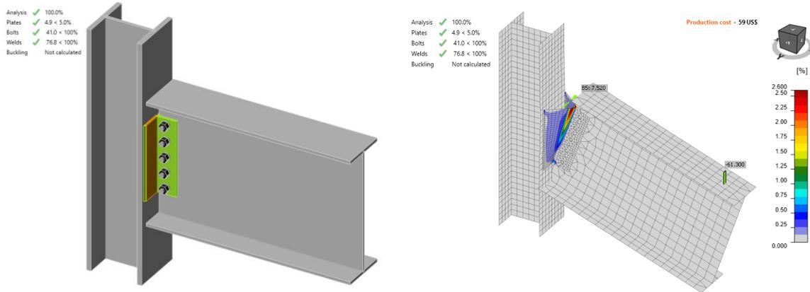
Figure C.4: IDEA StatiCa force applied on bolts in Test No. 9
