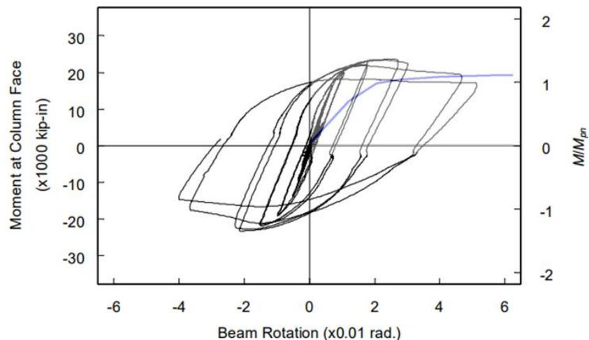
Figure 3.14: Comparison of the moment-rotation relationships of Test No. BFP measured during the experiment and calculated from IDEA StatiCa (blue line)
