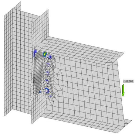
Figure C.8: IDEA StatiCa force applied on welding in Test No. 9
