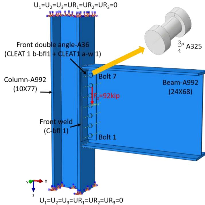
Figure 1.10: Model setup in ABAQUS
