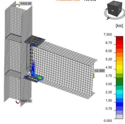
Figure K.10: IDEA StatiCa Model 9 and stress in contact distribution (LRFD)
