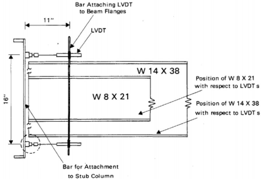
Figure 2.2: Measurements of horizontal displacements using the LVDT apparatus
