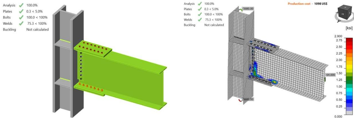
Figure K.8: IDEA StatiCa Model 7 and stress in contact distribution (LRFD)
