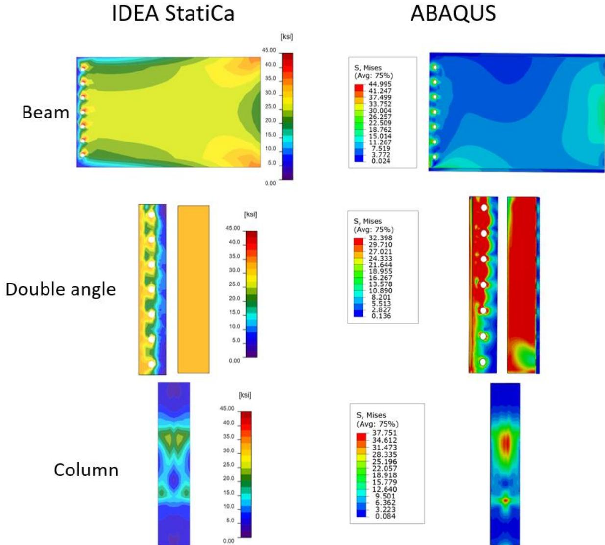
Figure D.1: Comparison of the predicted stress between IDEA StatiCa and ABAQUS for case 1
