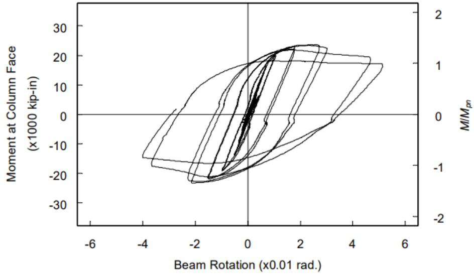
Figure 3.5: Applied load-beam tip displacement (Sato et al., 2007)
