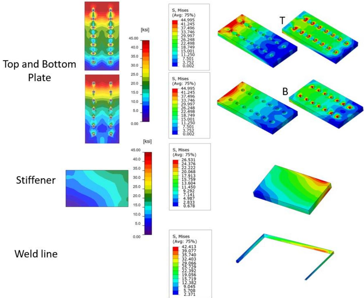
Figure L.1: Predicted stress between IDEA StatiCa and ABAQUS
