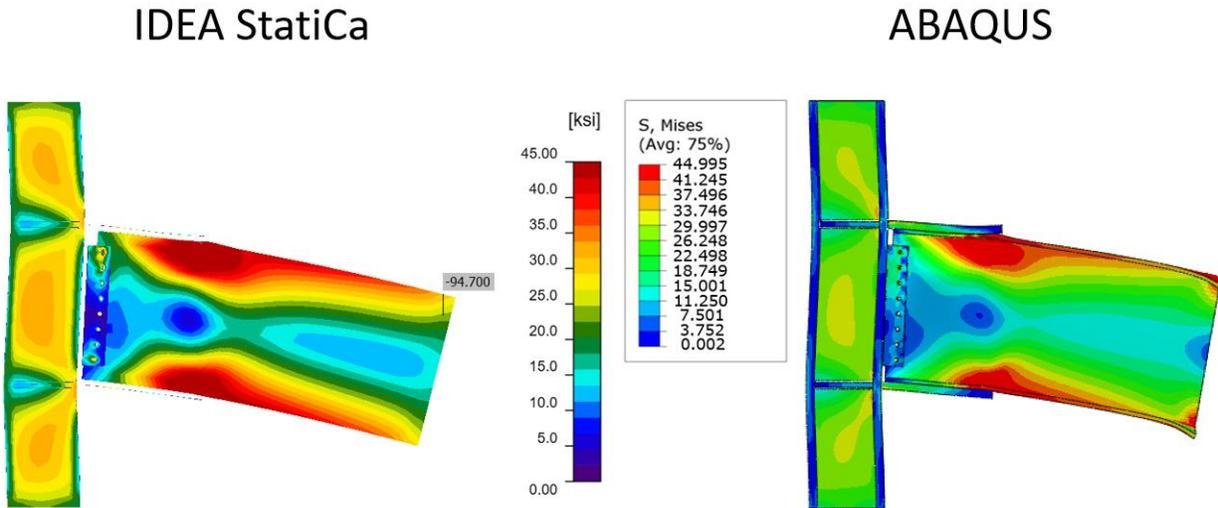
Figure 3.13: Side view comparison between IDEA StatiCa and ABAQUS with deformation scale factor of 20
