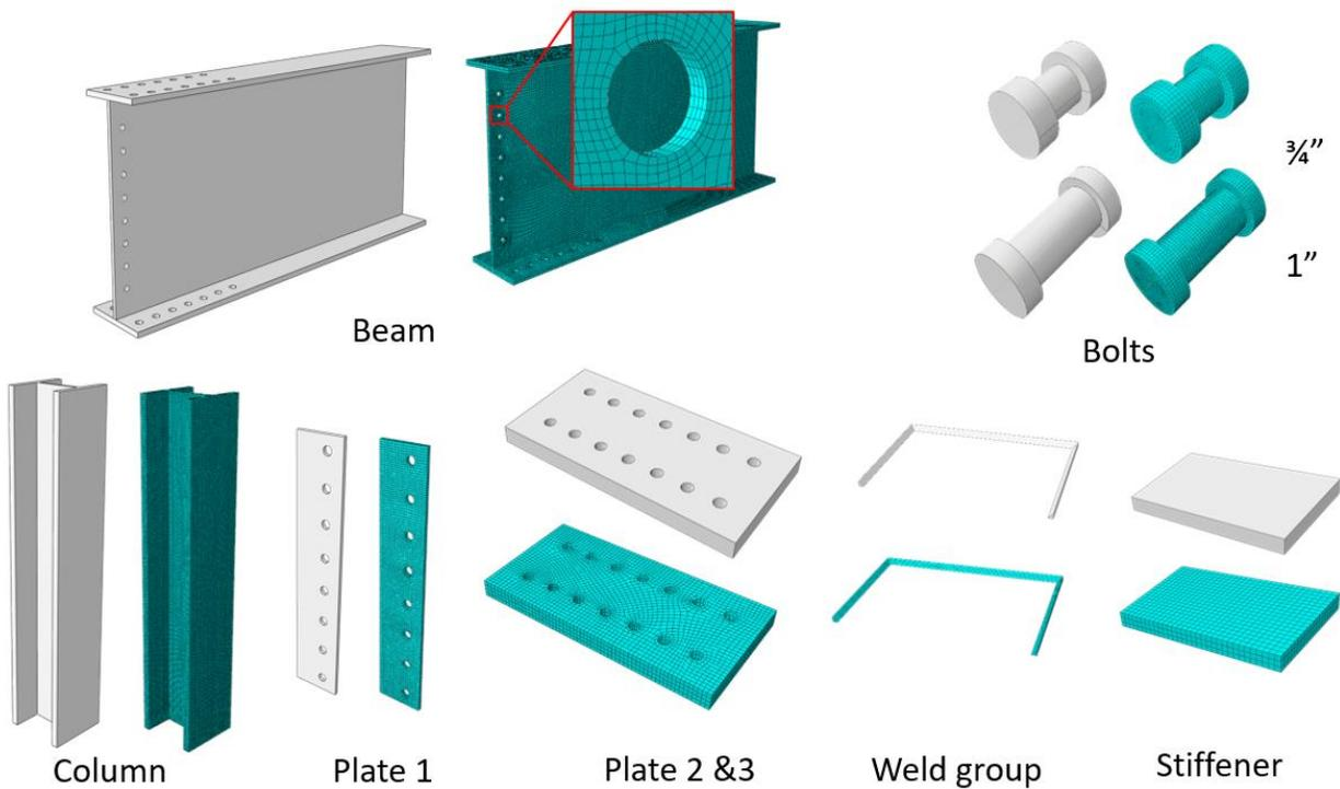
Figure 3.11: ABAQUS model mesh densities
