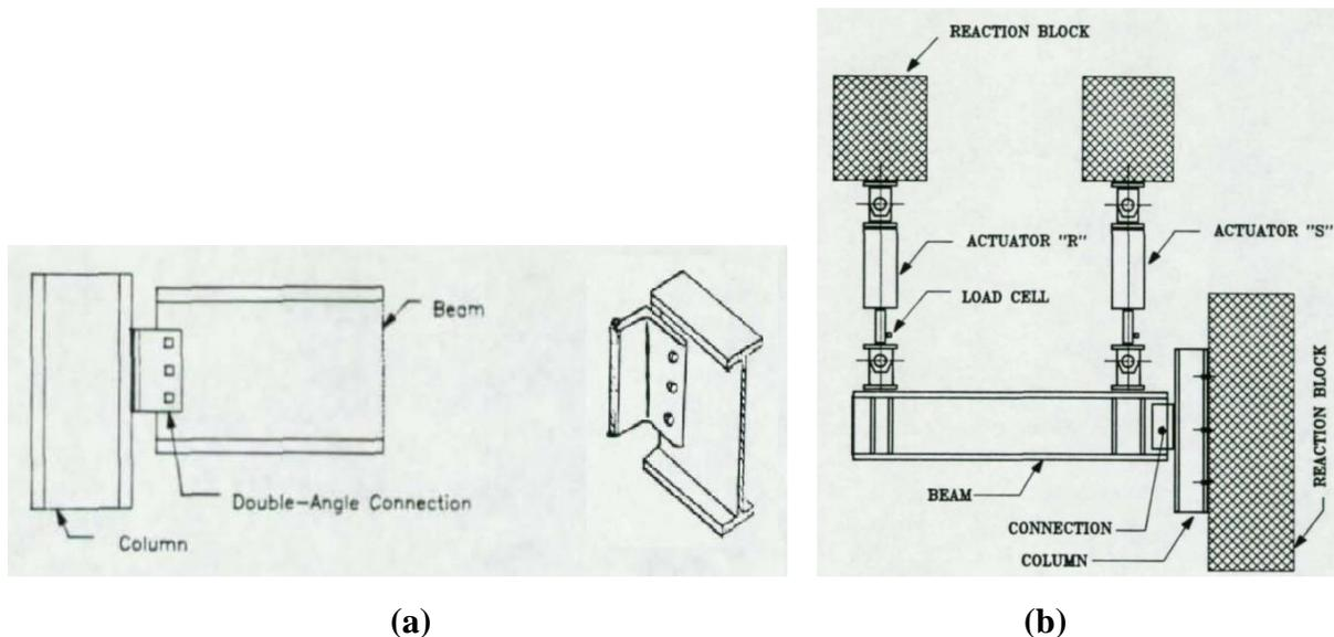
Figure 1.1: (a) Double angle connection specimens, and (b) test set-up (McMullin and Astaneh, 1988)
