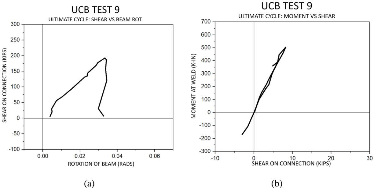
Figure 1.5: Test specimen No. 9: a) measured shear on connection-rotation of beam relationship, and b) moment at weld-shear on connection relationship
