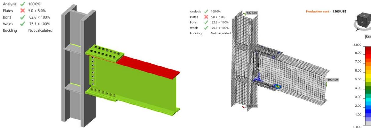
Figure K.6: IDEA StatiCa Model 5 and stress in contact distribution (LRFD)
