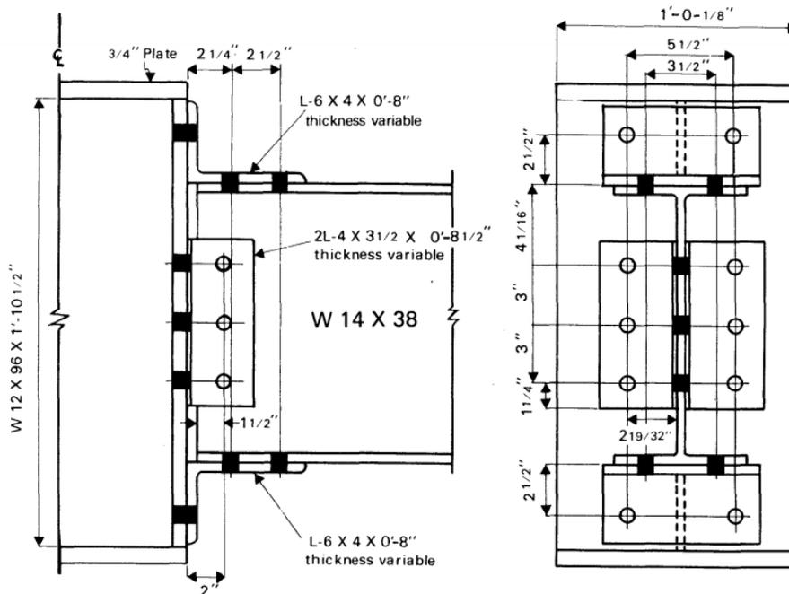
Figures 2.3: Details of connection for W14x38 beam
