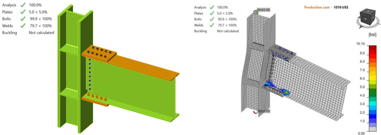
Figure K.9: IDEA StatiCa Model 8 and stress in contact distribution (LRFD)
