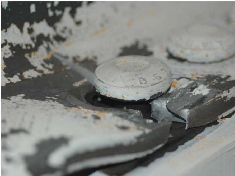
*Figure 3.8: Beam bottom flange net section fracture on 2nd cycle at +6% drift*
