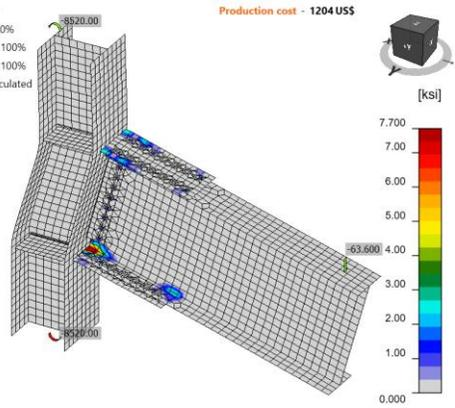
Figure K.11: IDEA StatiCa BFP and stress in contact distribution (ASD)
