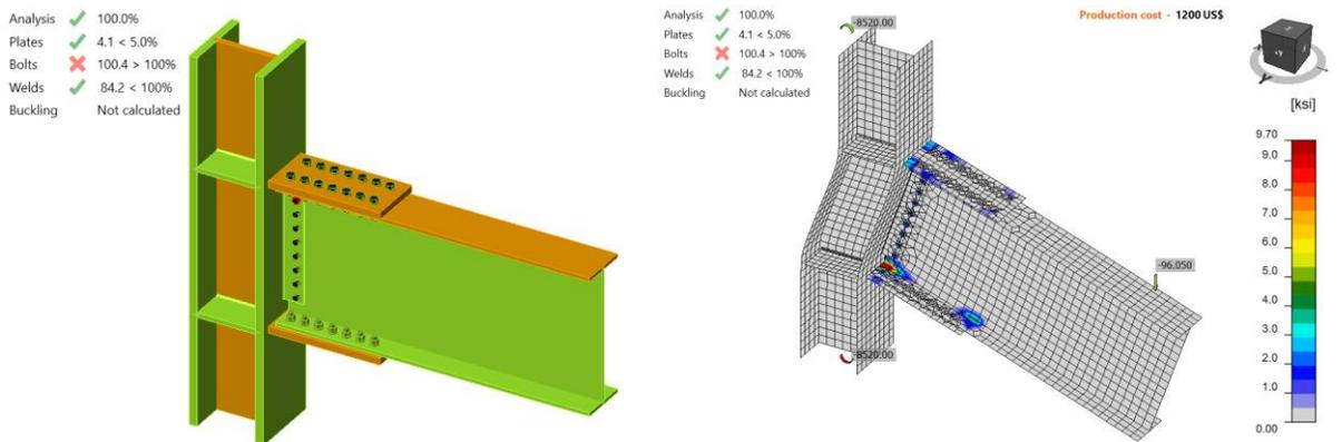
Figure K.2: IDEA StatiCa Model 1 and stress in contact distribution (LRFD)
