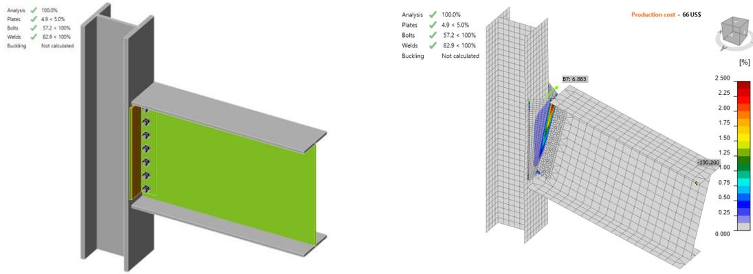
Figure C.1: IDEA StatiCa force applied on bolts in Test No. 4
