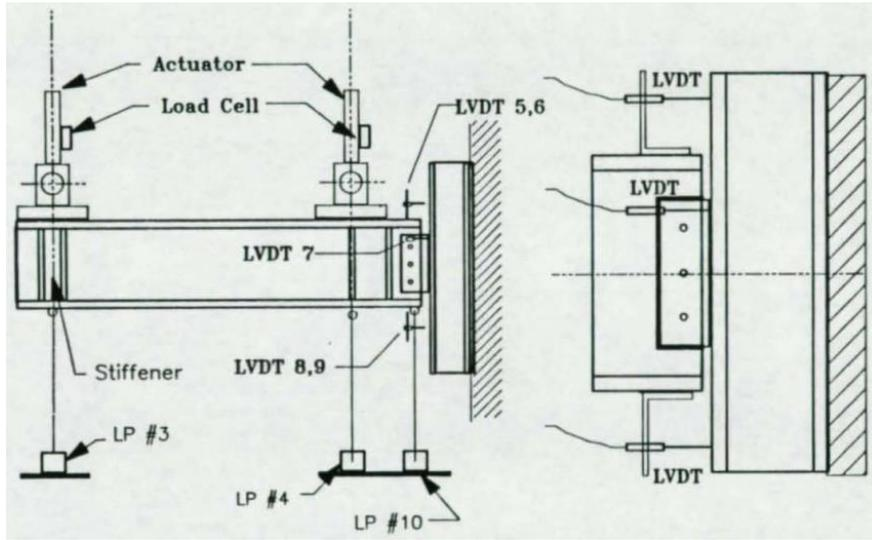
Figure 1.6: Diagram of the instrumentation used during the experiment (McMullin and Astaneh, 1988)
