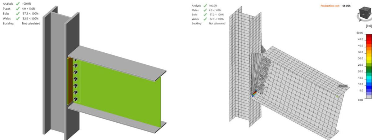
Figure C.12: IDEA StatiCa force applied on bolts in Model 4
