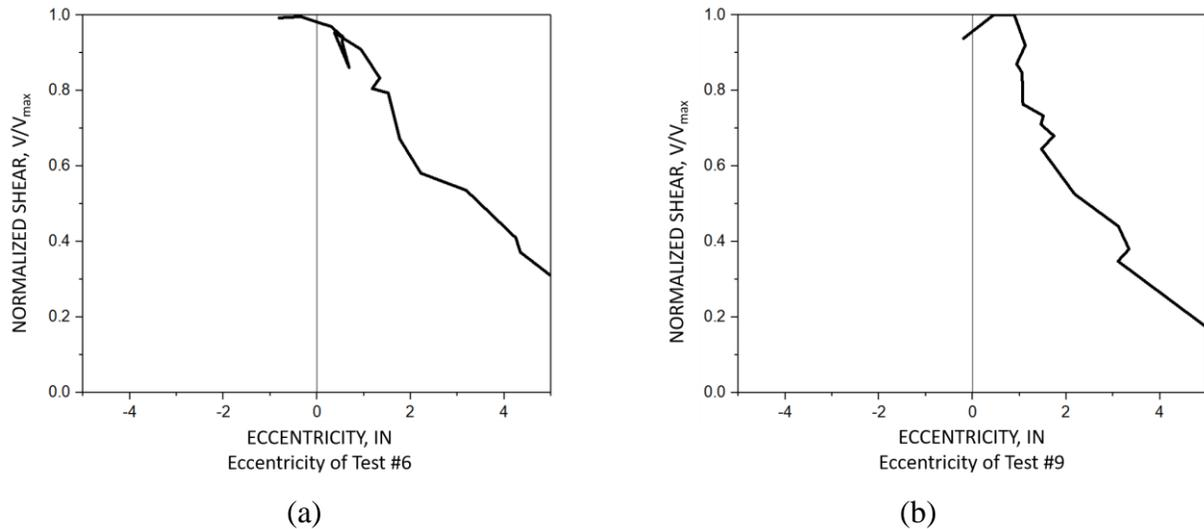
Figure 1.8: (a) Normalized shear-eccentricity of Test No 6, and (b) Normalized shear-eccentricity of Test No 9 (McMullin and Astanteh, 1988)
