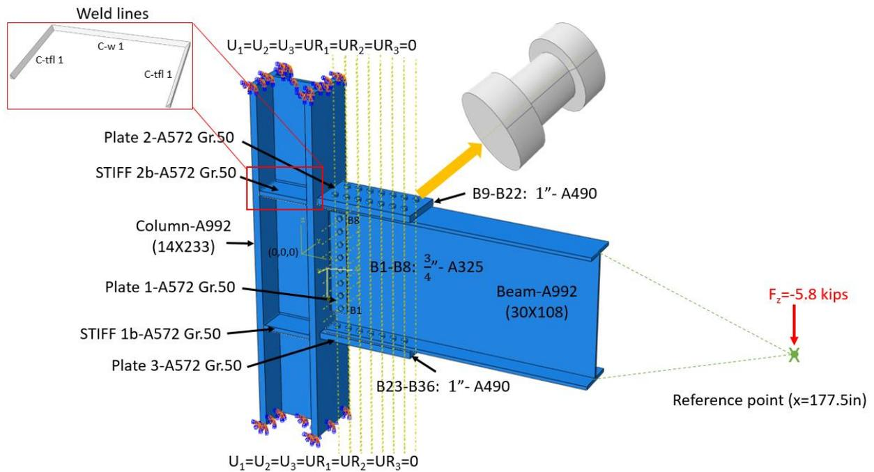
Figure 3.10: Model setup in ABAQUS
