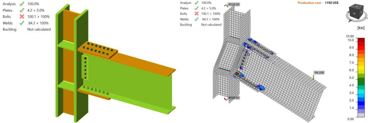
Figure K.4: IDEA StatiCa Model 3 and stress in contact distribution (LRFD)
