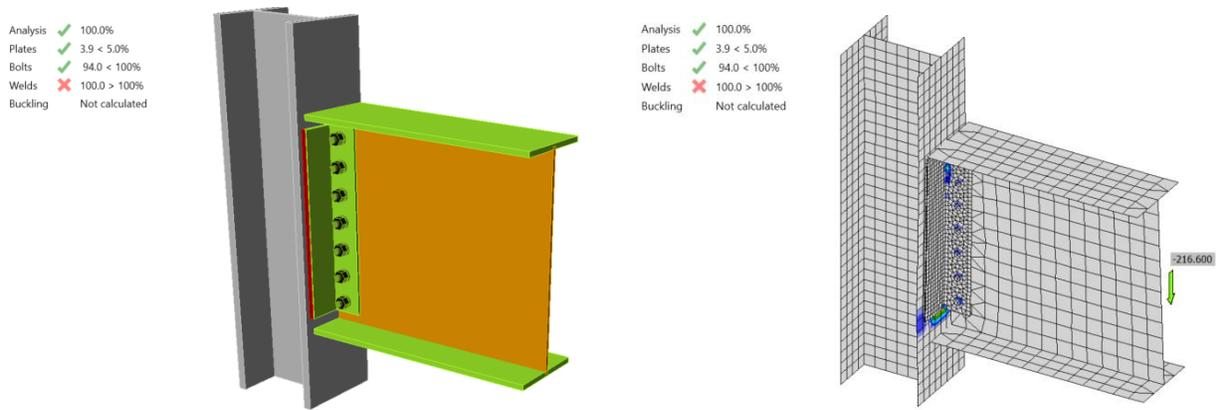
Figure C.5: IDEA StatiCa force applied on welding in Test No. 4
