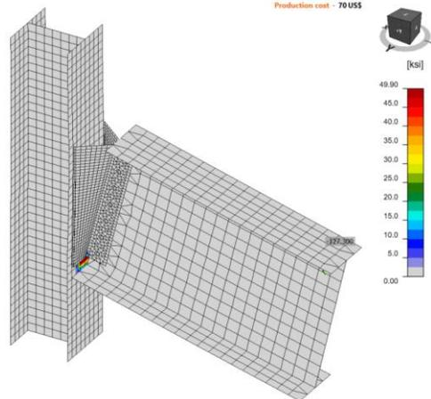
Figure C.9: IDEA StatiCa force applied on bolts in Model 1
