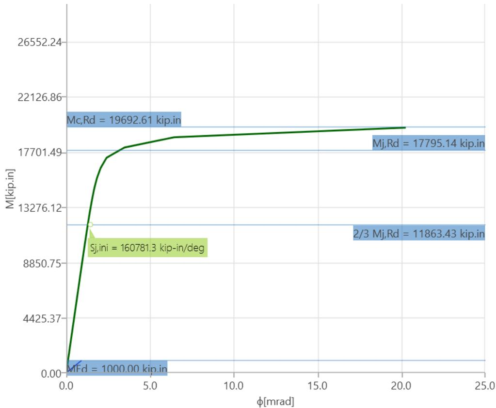
Figure 3.9: Moment-rotation relationship for Test No. BFP (IDEA StatiCa)
