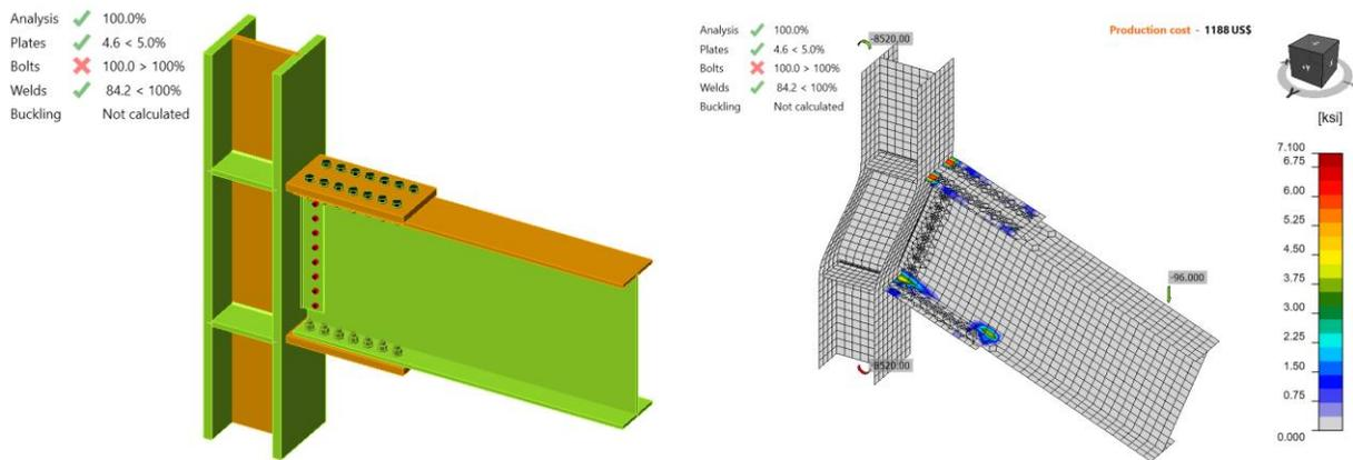
Figure K.3: IDEA StatiCa Model 2 and stress in contact distribution (LRFD)
