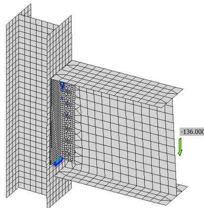
Figure C.17: IDEA StatiCa force applied on welding in Model 3
