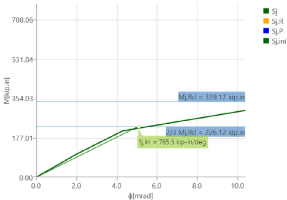
Figure 2.10: Moment-rotation relationship for Test No. 14S1 computed by IDEA StatiCa
