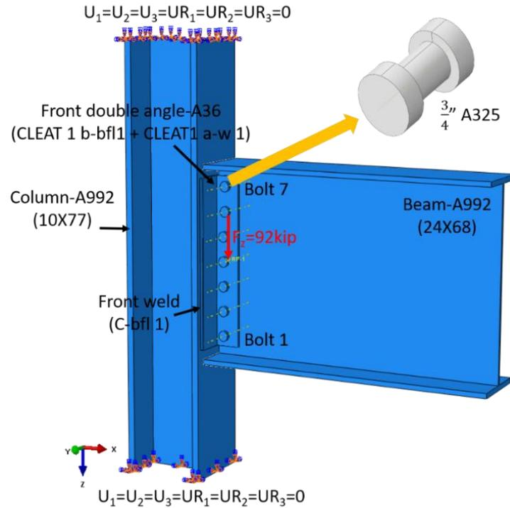
Figure 1.10: Model setup in ABAQUS
