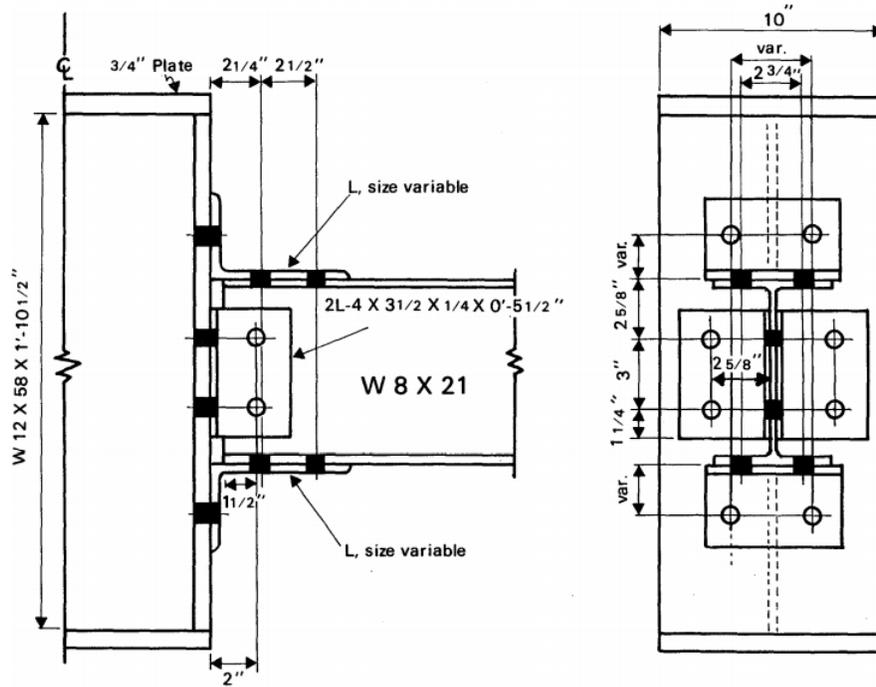
Figures 2.4: Details of connection for W8x21 beam
