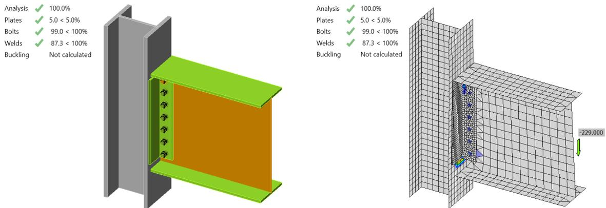
Figure C.15: IDEA StatiCa force applied on welding in Model 1
