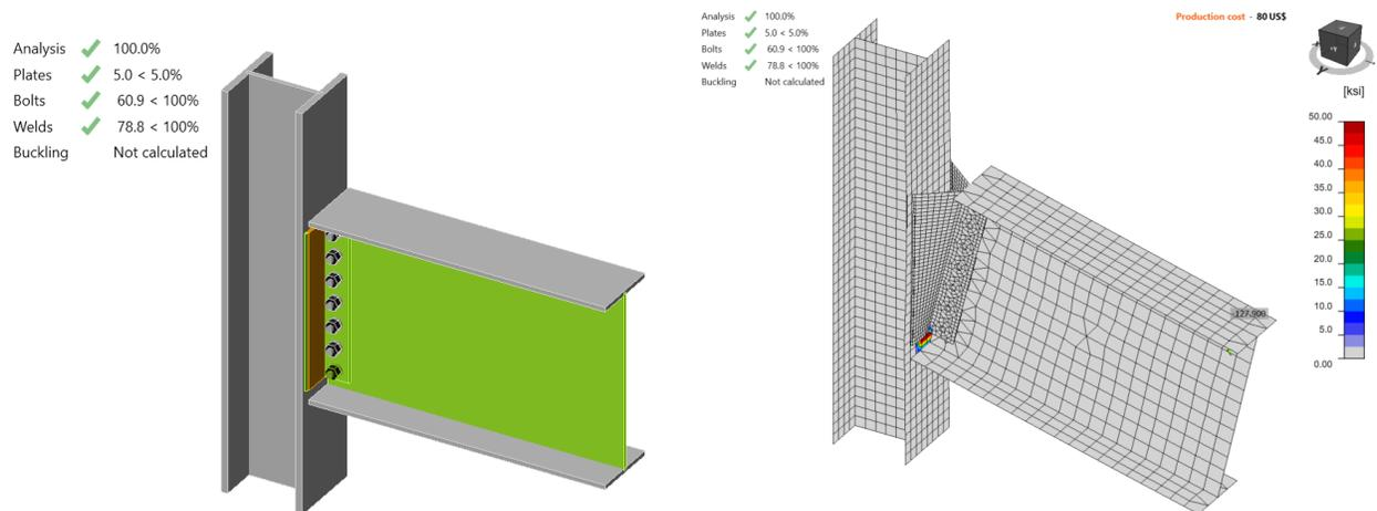
Figure C.14: IDEA StatiCa force applied on bolts in Model 6
