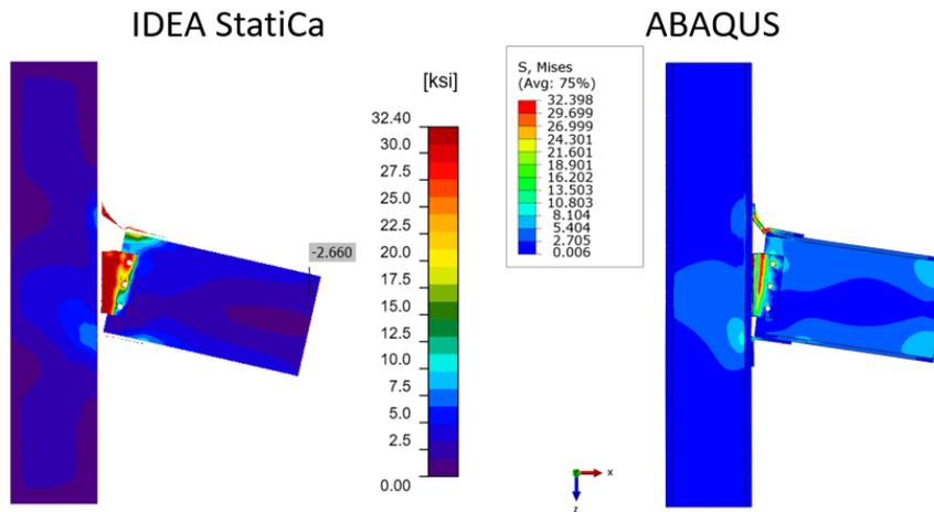
Figure 2.14: Side view comparison between IDEA StatiCa and ABAQUS with deformation scale factor of ten
