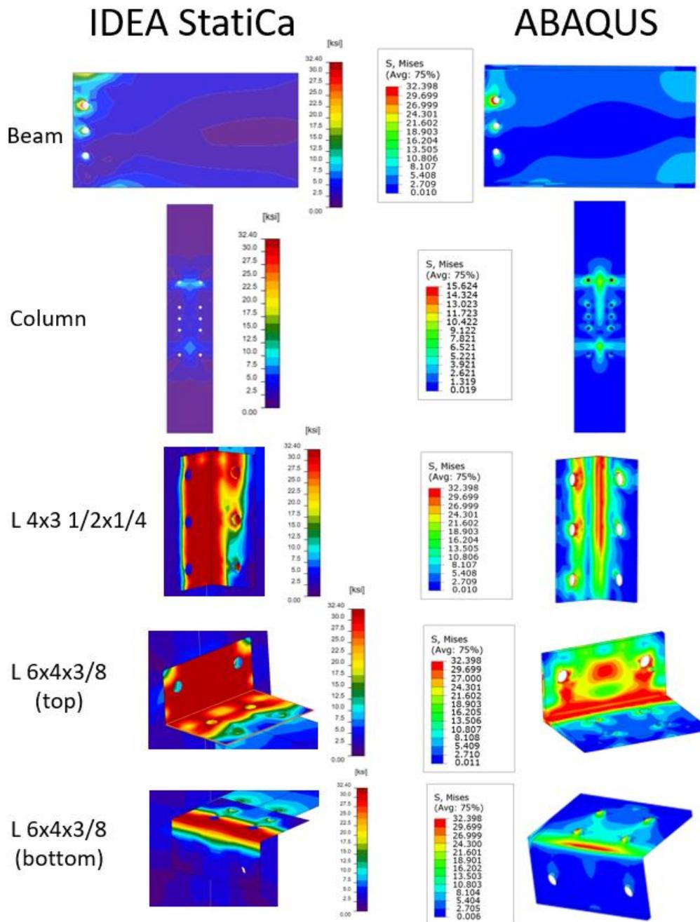
Figure H.1: Predicted stress between IDEA StatiCa and ABAQUS
