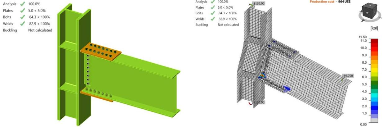
Figure K.7: IDEA StatiCa Model 6 and stress in contact distribution (LRFD)
