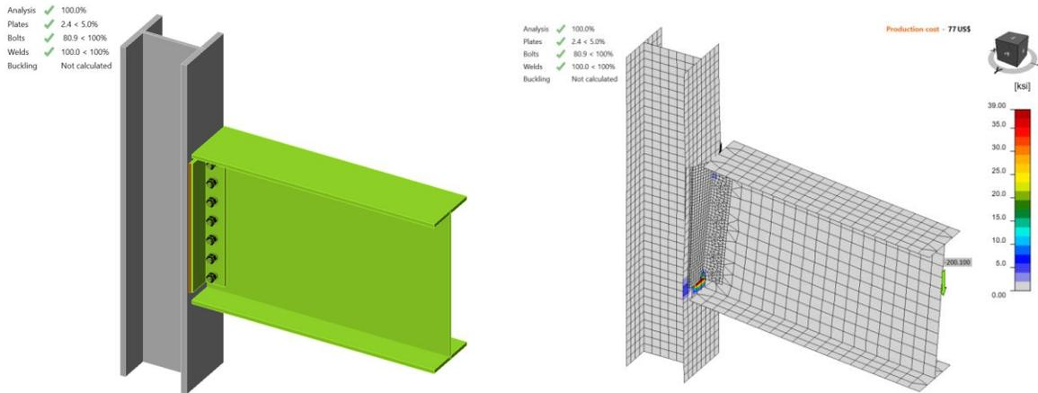
Figure C.10: IDEA StatiCa force applied on bolts in Model 2
