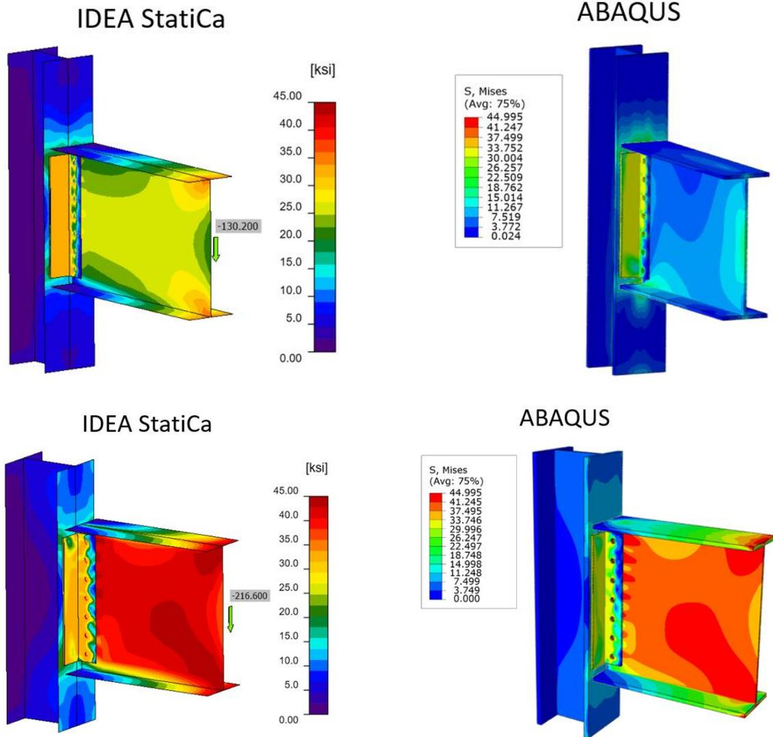
Figure 1.12: Predicted von Mises stress between IDEA StatiCa and ABAQUS models; case 1 (top row): shear load was applied on the centroid of the bolt group, and case 2 (bottom row): shear load was applied on the weld lines
