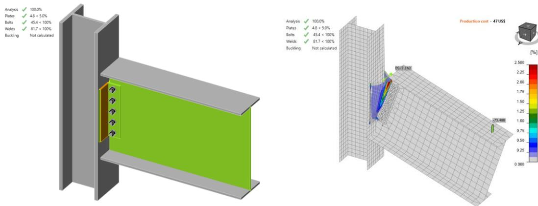
Figure C.2: IDEA StatiCa force applied on bolts in Test No. 5
