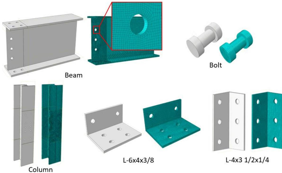
Figure 2.12: ABAQUS model mesh densities
