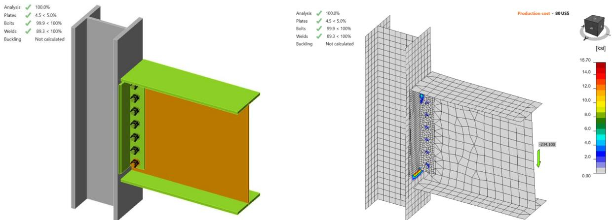
Figure C.20: IDEA StatiCa force applied on welding in Model 6
