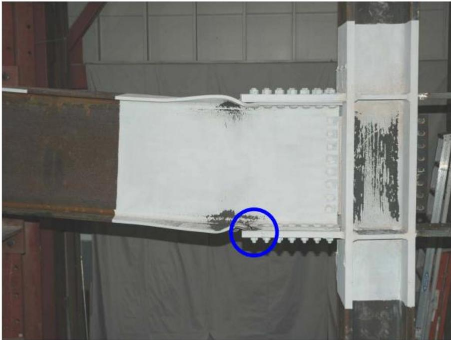
*Figure 3.7: Fracture location (Sato et al., 2007)*
