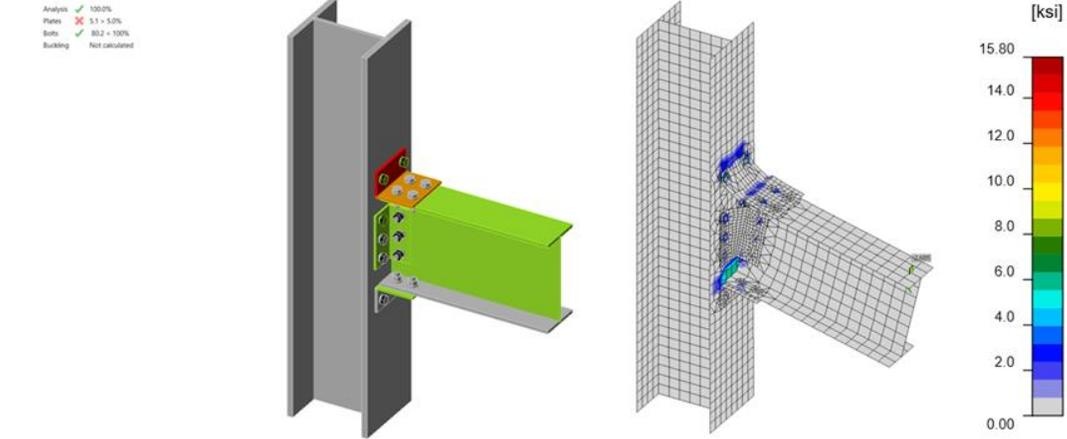
Figure G.1: IDEA StatiCa Test No. 14S1 (LRFD)
