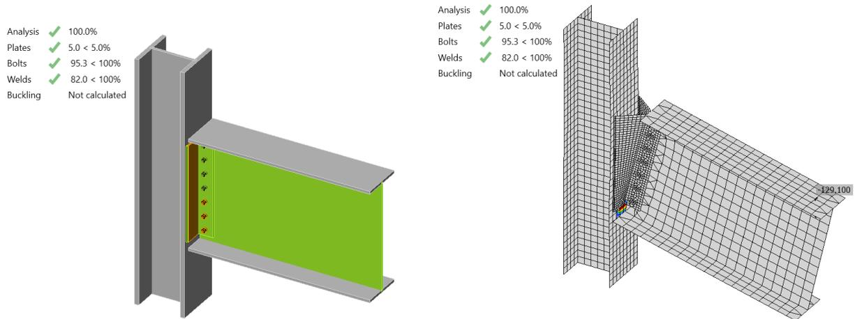
Figure C.11: IDEA StatiCa force applied on bolts in Model 3
