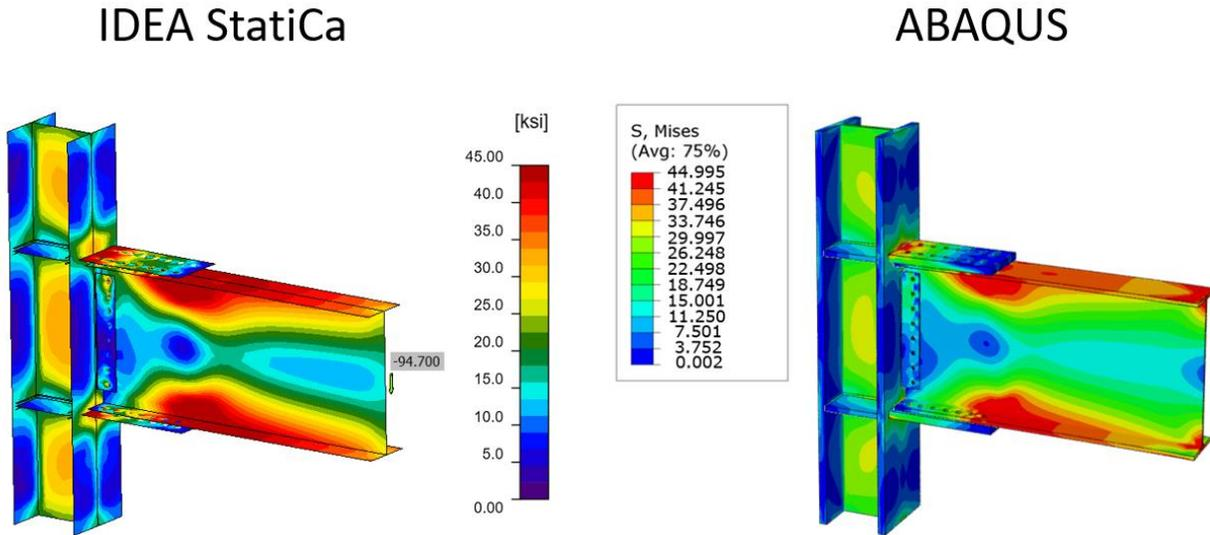
Figure 3.12: Comparison of the predicted von-Mises stress between IDEA StatiCa and ABAQUS
