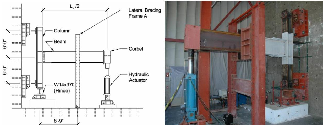
Figure 3.1: Test Setup: (a) schematic; (b) photo (Sato et al., 2007)
