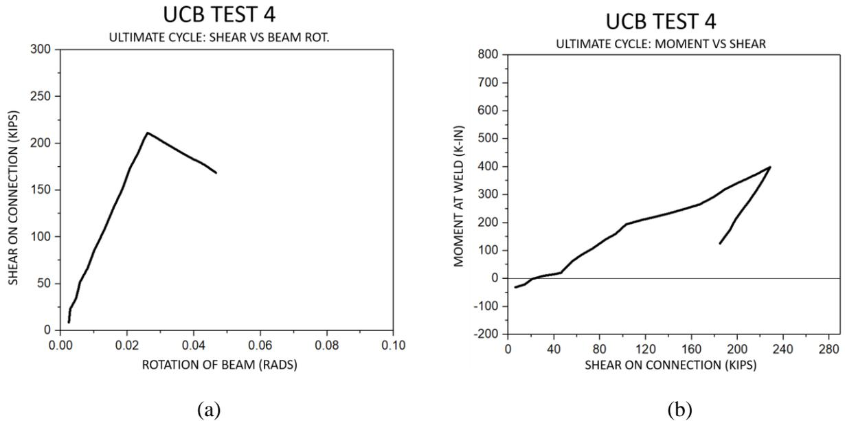
Figure 1.2: Test specimen No. 4: a) measured shear on connection-rotation of beam relationship, and b) moment at weld-shear on connection relationship
