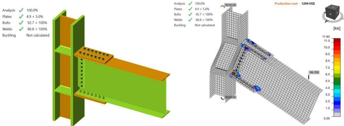
Figure K.1: IDEA StatiCa BFP and stress in contact distribution
