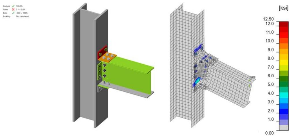
Figure G.11: IDEA StatiCa Test No. 14S1 (ASD)
