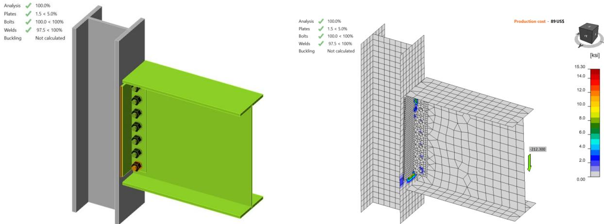
Figure C.19: IDEA StatiCa force applied on welding in Model 5
