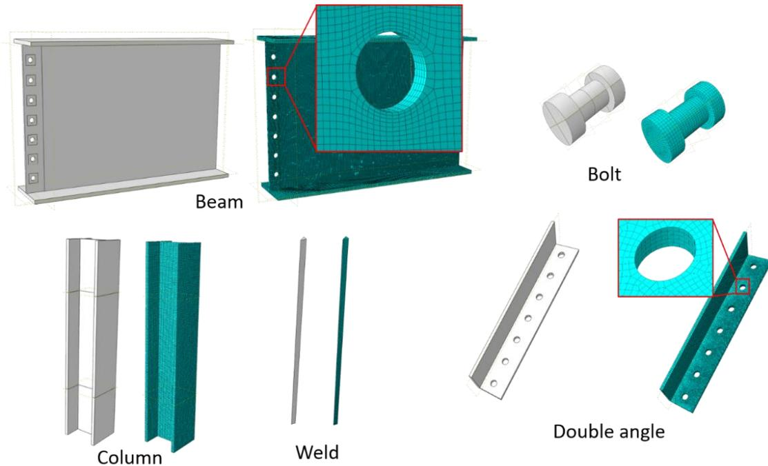
*Figure 1.11: ABAQUS model mesh densities*
