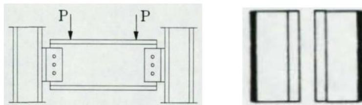
Figure A.1: (a) Test setup, and (b) connection detail of Test No. 4 (McMullin and Astaneh, 1988)
