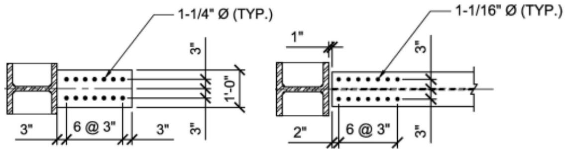
Figure 3.4: Bolt schedule details for the specimen No. BFP: (a) flange plate; and (b) beam flange (Sato et al., 2007)
