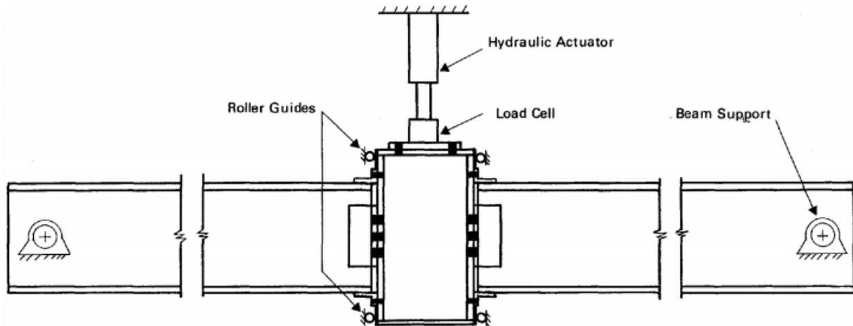
Figure 2.1: Test set-up used by Azizinamini et al. (1985)
