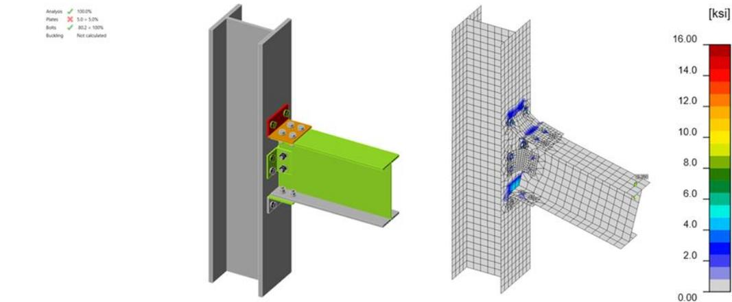
Figure G.3: IDEA StatiCa Test No. 14S3 (LRFD)
