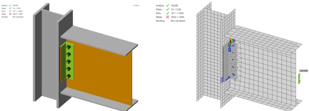
Figure C.6: IDEA StatiCa force applied on welding in Test No. 5
