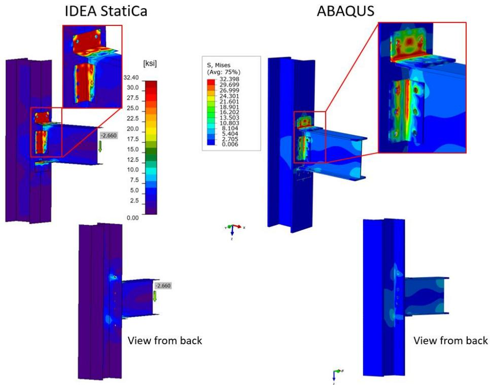
Figure 2.13: Comparison of the predicted von-Mises stress between IDEA StatiCa and ABAQUS
