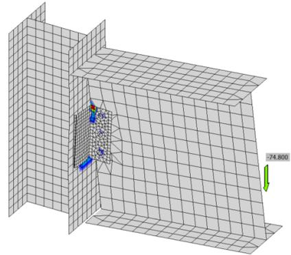
Figure C.7: IDEA StatiCa force applied on welding in Test No. 6
