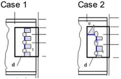
>    R<sub>n</sub> = 0,6F<sub>y</sub>A<sub>gv</sub> + U<sub>bs</sub>F<sub>u</sub>A<sub>nt</sub> = 297 kN
