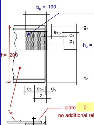
**fin plate thickness d = 10 mm**
