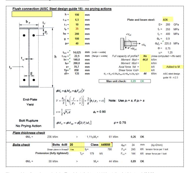
The resulting force in one bolt is: **Ft** =  $M_u / (2 d_1) = 44 \text{ kNm} / (2 \text{ x } 0.135 \text{m}) =$ **163 kN**
