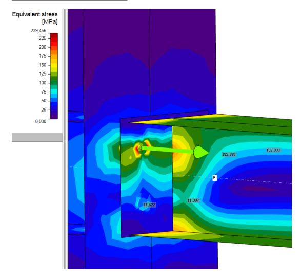
The tension force in upper bolt is Ft = 152.4 kN
