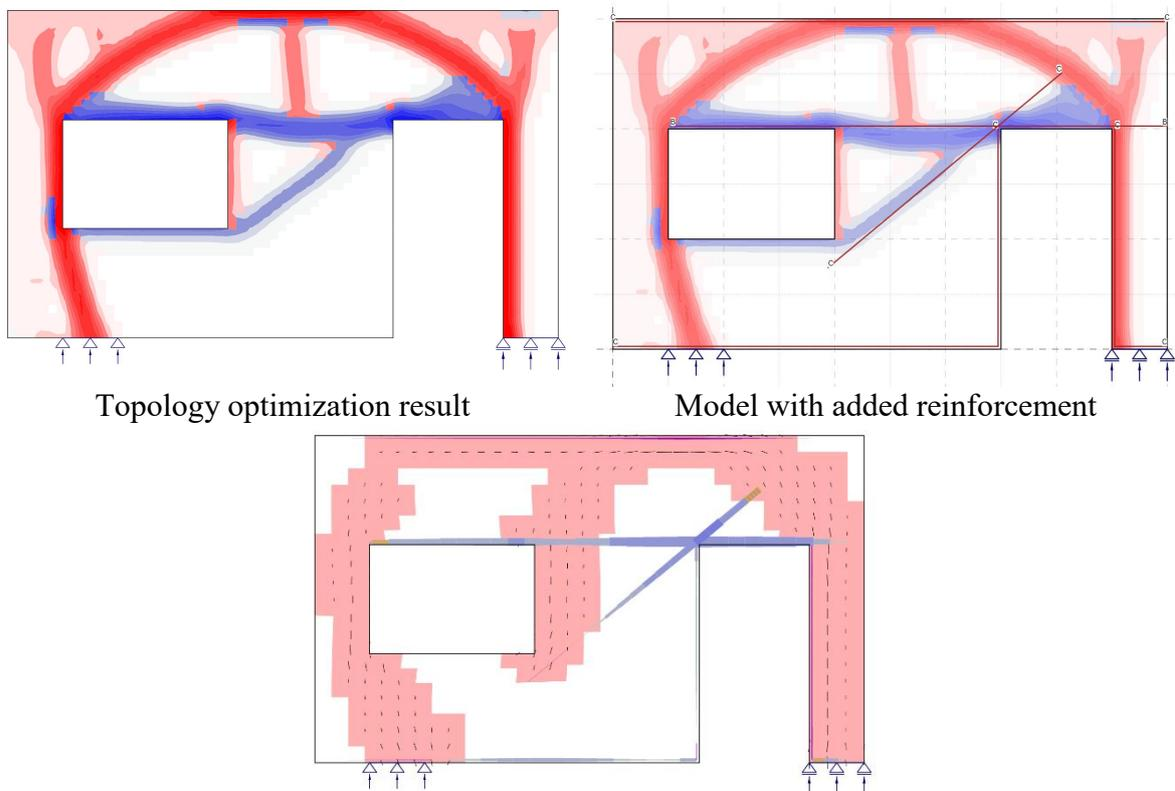
Result of non-linear analysis, red – stress in compressed concrete, blue – forces in reinforcement bars
