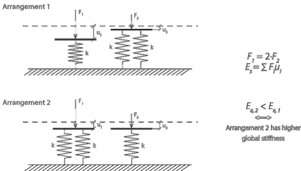
**Figure 2 Strain energy in two systems with the same amount of material**
