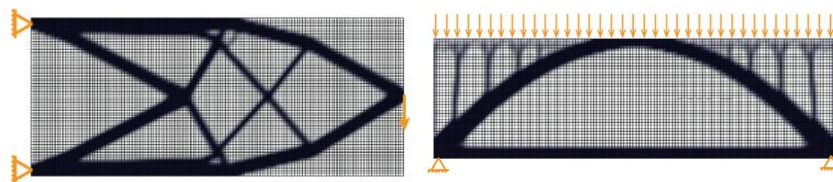
**Figure 5** Load-carrying structure of cantilever and beam
