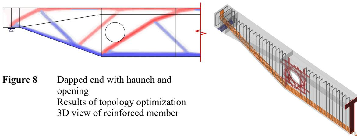
**Figure 8** Dapped end with haunch and opening
