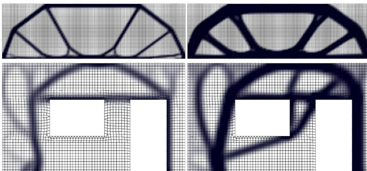
**Figure 4** Low and significant effects of effective volume on generated geometry
