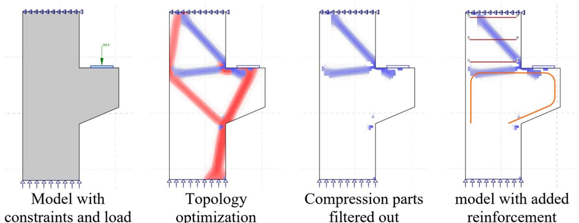
Figure 6 Reinforcement of a bracket
