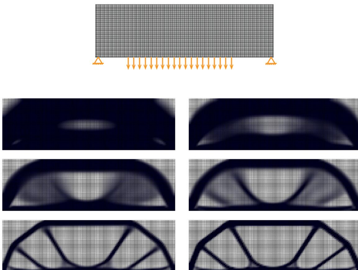
**Figure 3** Gradual convergence of a vertically loaded structure with two point supports, iterations 1, 3, 7, 10, 15 and 19
