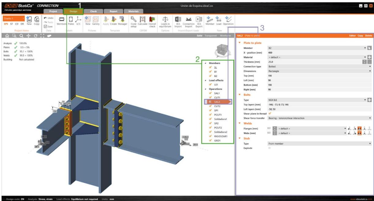
Figure Error! No text of specified style in document..14. Workflow example with the *Operation* item.
