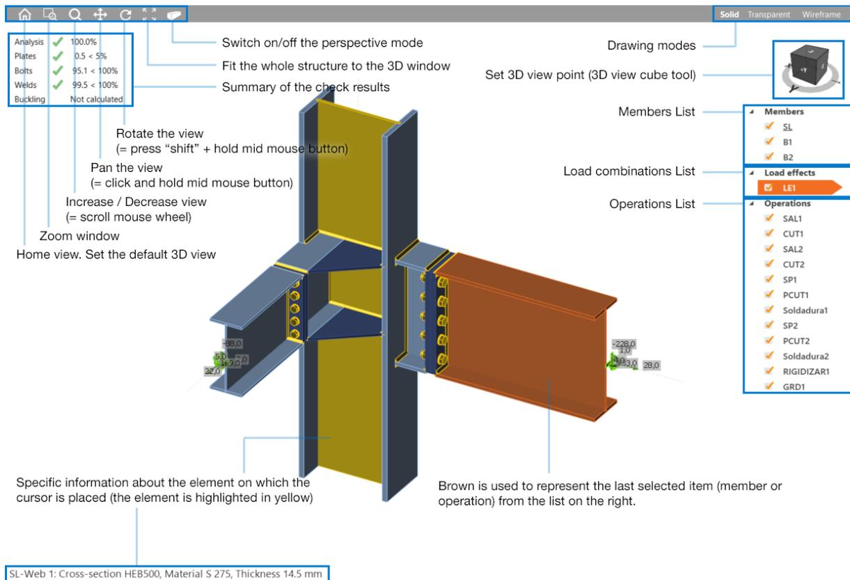
Figure Error! No text of specified style in document..10. Appearance and description of the graphic window.
