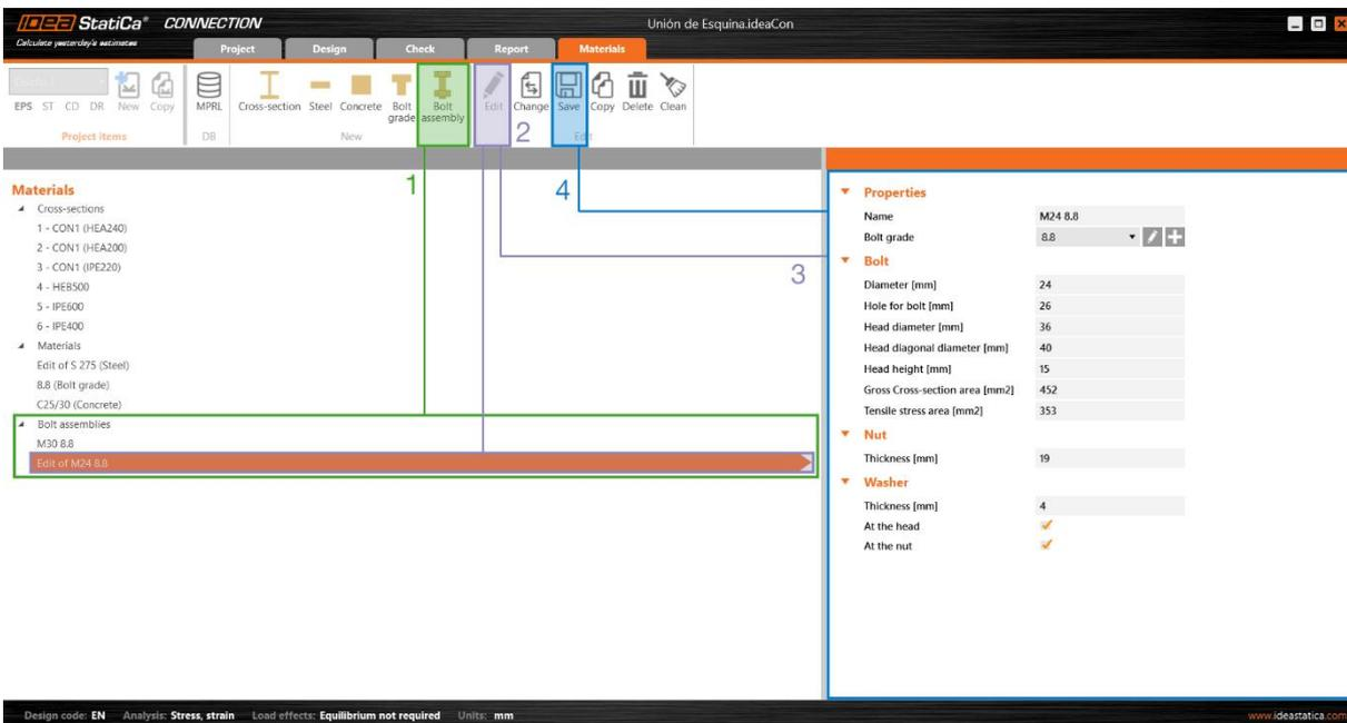
Figure Error! No text of specified style in document..18. Specification of the features of customized bolts.
