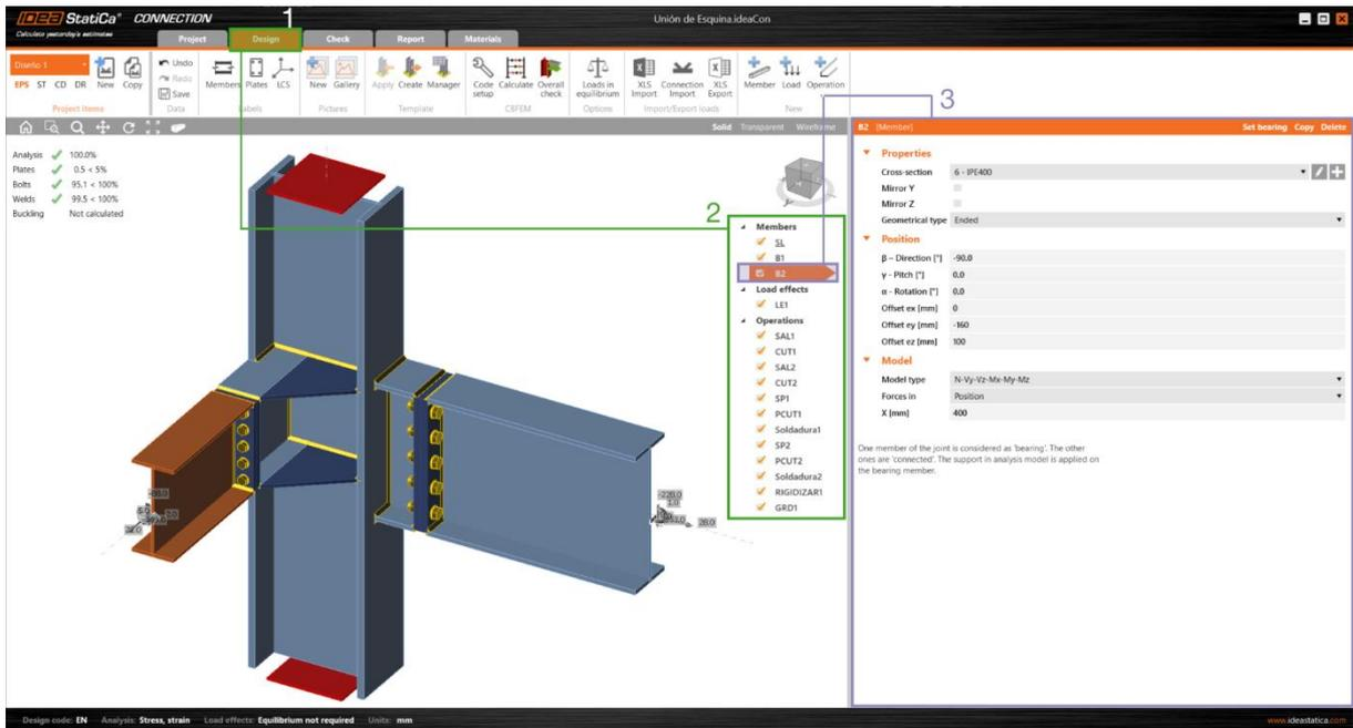
Figure Error! No text of specified style in document..13. Workflow example with the *Member* item.
