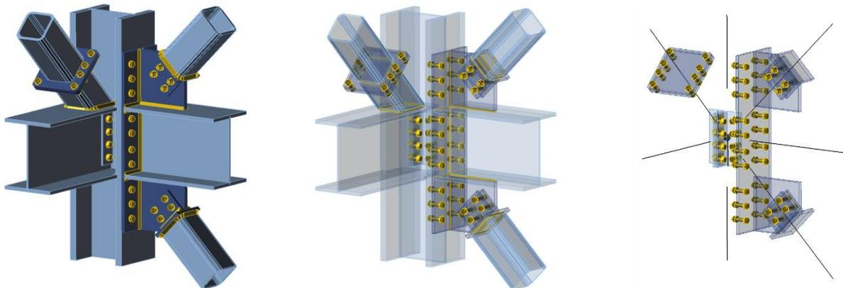
Figure Error! No text of specified style in document..11. Configurations of the view of the connection. Solid, transparent and wireframe.
