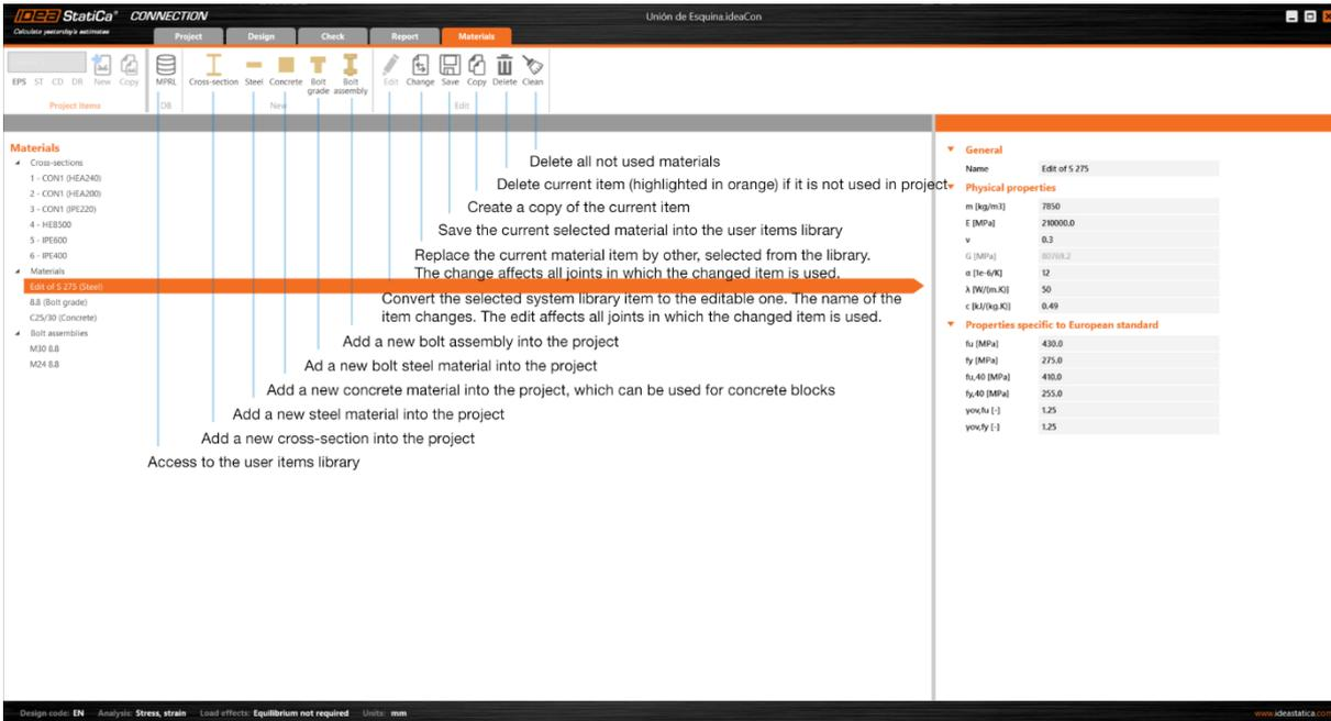
Figure Error! No text of specified style in document..17. Specification of customized materials
