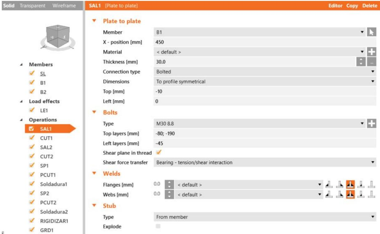
Figure Error! No text of specified style in document..12. General appearance of the Data and Features Entry tab.
