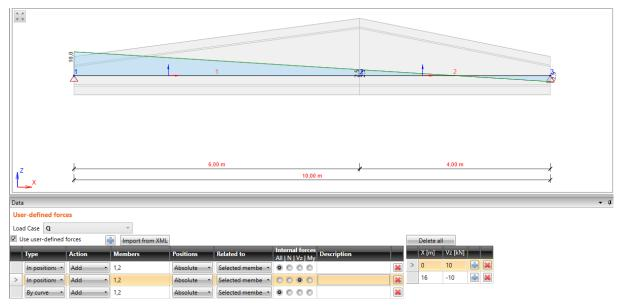
Current load case can be set in the list **Load cases**. User defined internal forces already defined in the current load case are displayed in the table.
