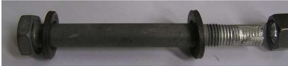
Sample 4: Stripping of the bolt threads
