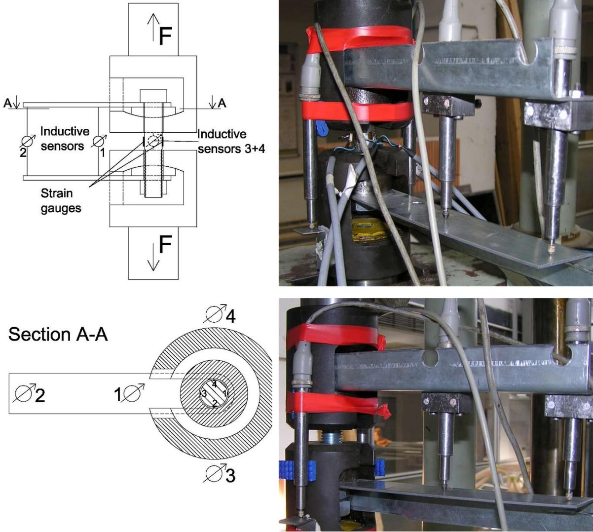
Fig. 12: Scheme of the measuring instruments
