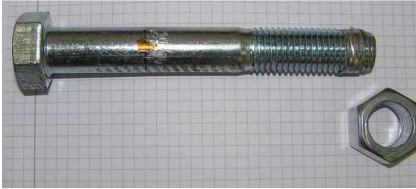
Sample 1: Stripping of the nut threads
