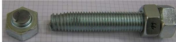
Sample 11: Rupture of the bolt close to the head
