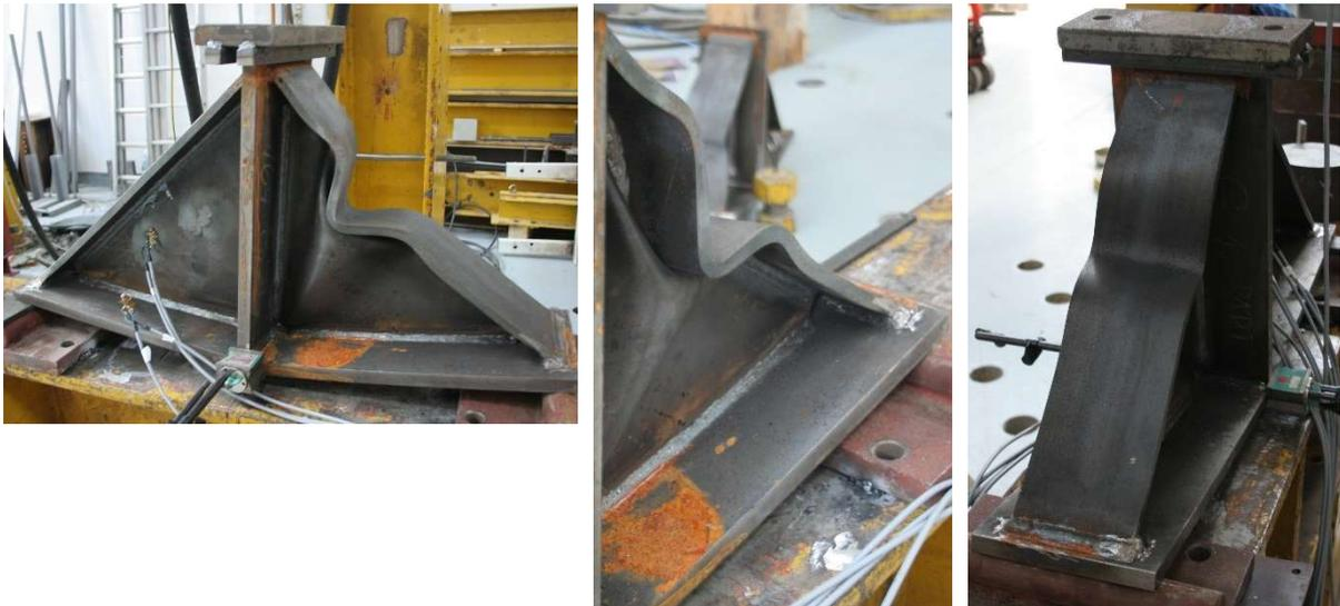
**Fig. 7: Sample F after the test**
