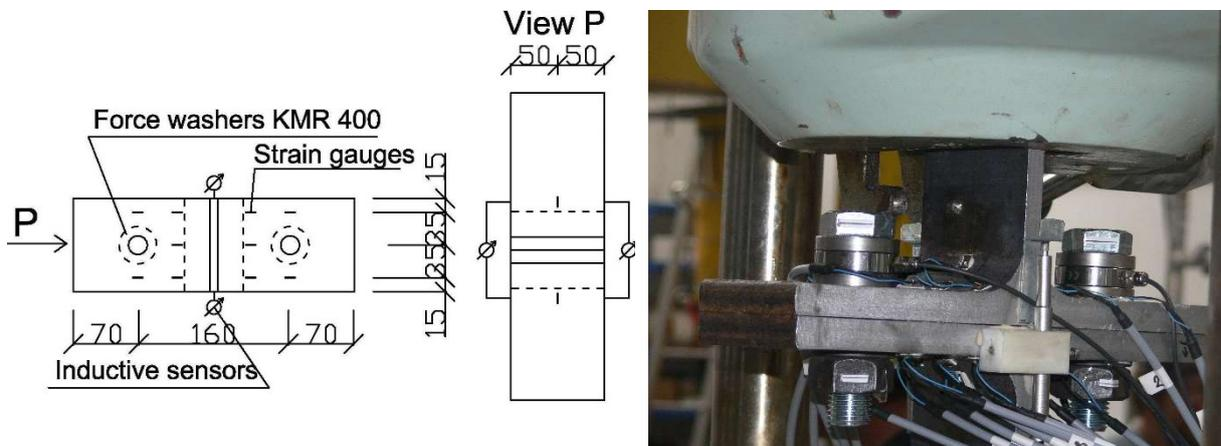
Fig. 14: Scheme of the T-stub experiment.
