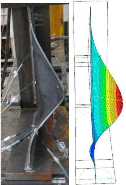
Fig. 9: Sample B - comparison of the deformed shape and numerical model
