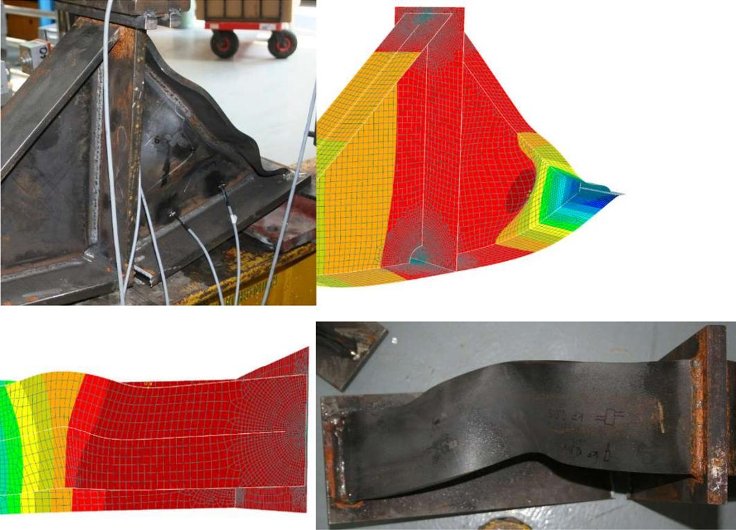
Fig. 11: Sample E - comparison of the deformed shape and numerical model
