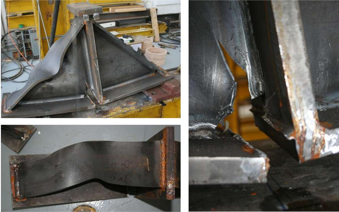
**Fig. 6: Sample E after the test**
