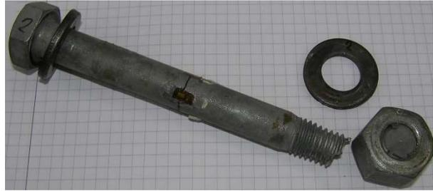
Sample 2: Rupture of the bolt close to the nut
