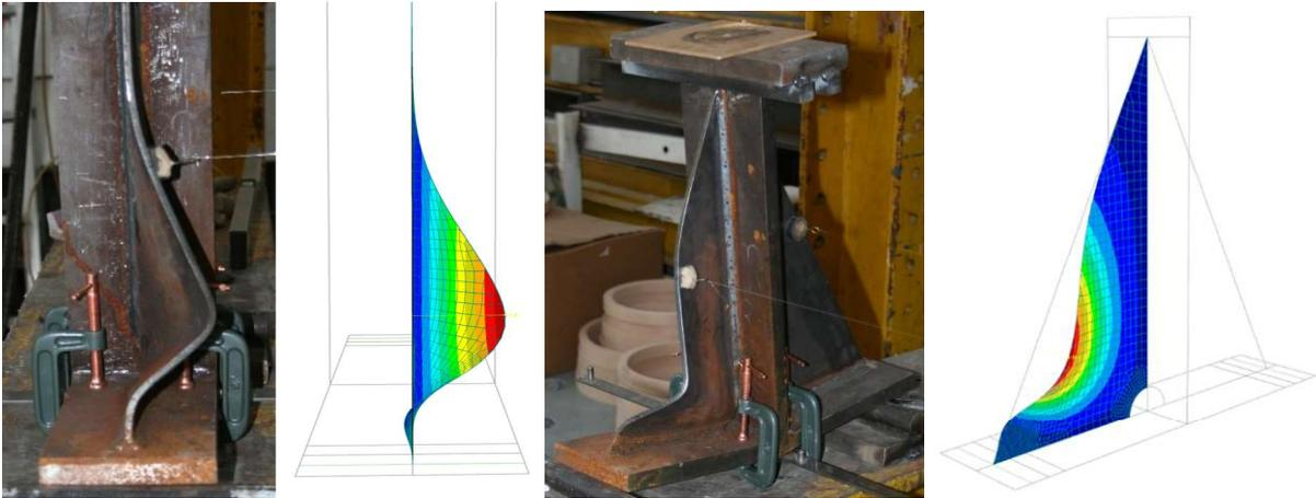
Fig. 8: Sample A - comparison of the deformed shape and numerical model
