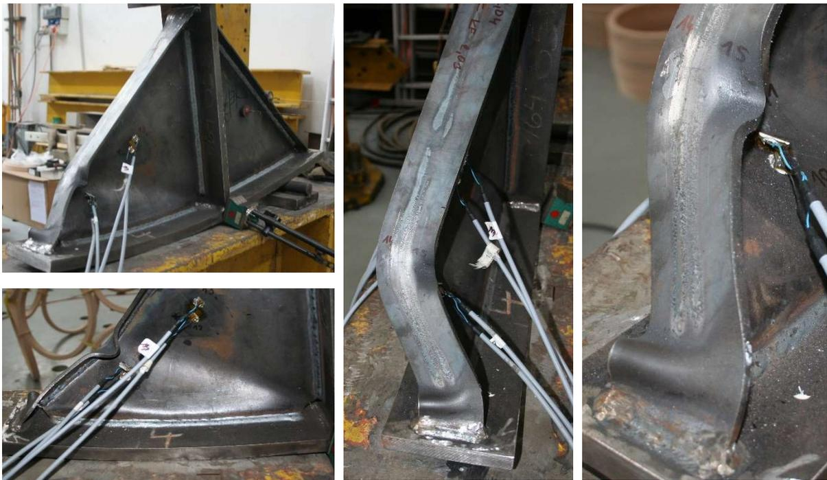
Fig. 5: Sample D after the test
