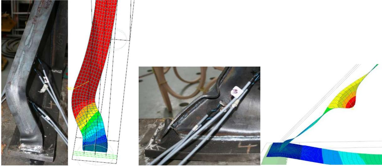
Fig. 10: Sample D - comparison of the deformed shape and numerical model
