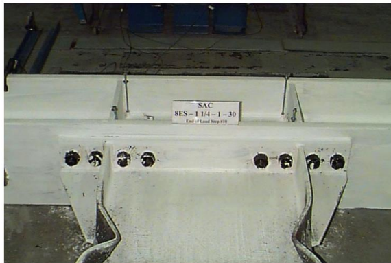
Figure 2.7: Left) Variation 3 after testing; Right) moment-total plastic rotation relationship (Sumner et al., 2000)
