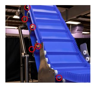
**STEP 5:** Add all recorded measurements to calculate the length of your existing belt.
