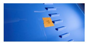
**STEP 4:** Repeat this process to move the starting point through the entirety of the belt circuit until you return to your first mark.
