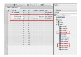
**Note:** it is required to put "OUT 32 WORD" at slot 1 and "IN 32 WORD" at slot 2. Otherwise, it does not work
