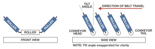
Figure 66: Tilt angles and direction of belt travel
