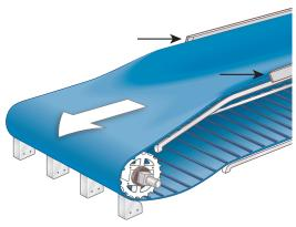
Use UHMW-PE containment rails or blocks for lateral belt containment. See Belt Containment.
