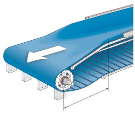
Ensure the transition distance (distance from end of troughed conveyor to drive or idle shaft center) is adequate. The transition distance must be a minimum of 1.5 times the belt width. Proper transition distance minimizes strain on belt edges and reduces belt friction.
