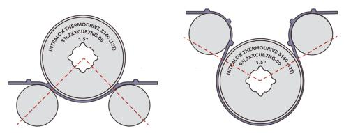
Figure 71: 90-degree and 225-degree belt-to-sprocket engagement
