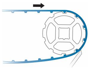
Figure 56: Scraper mounted at an angle
