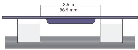
Figure 75: Single lug between containment rails
