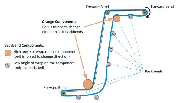
Figure 7: Sidewall backbends
