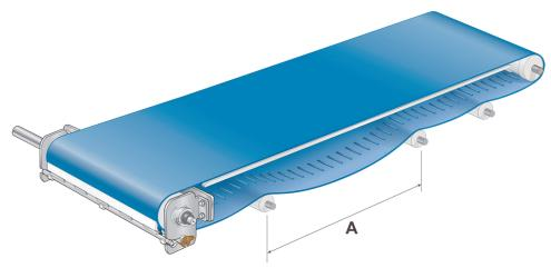
Figure 68: Correct support spacing
