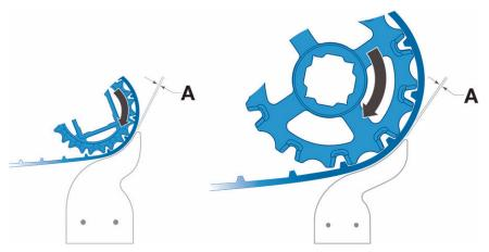
A 0.005–0.05 in (0.13–1.25 mm) spacing Figure 49: Correct limiter placement
