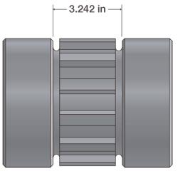
Figure 73: Sprocket inner dimensions
