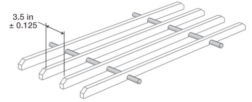
Figure 76: Gap dimensions between containment rails
