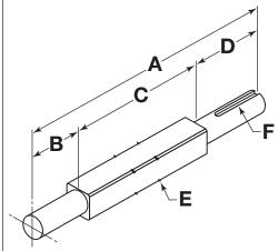
Figure 45: Square drive shaft components
