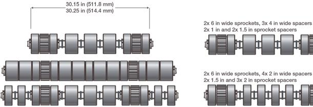
Figure 4: Drive sprocket and idle roller spacing
