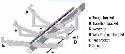
Figure 18: Trough converter components
