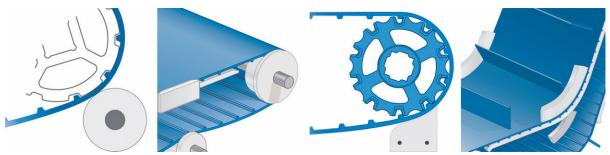
Figure 24: Components at or above the minimum bend radius
