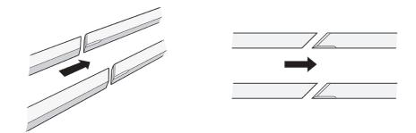
Figure 31: Rails chamfered at a 45-degree angle
