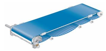
Figure 37: Catenary sag between components
