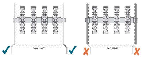
Figure 39: Correct steel brakes clearance
