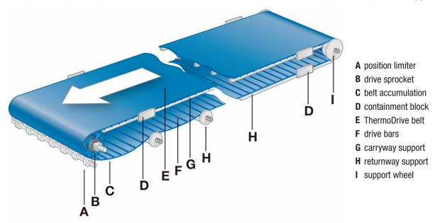
Figure 26: Conveyor belt components
