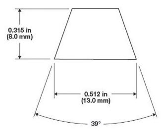
Figure 8: V-guide nominal geometry
