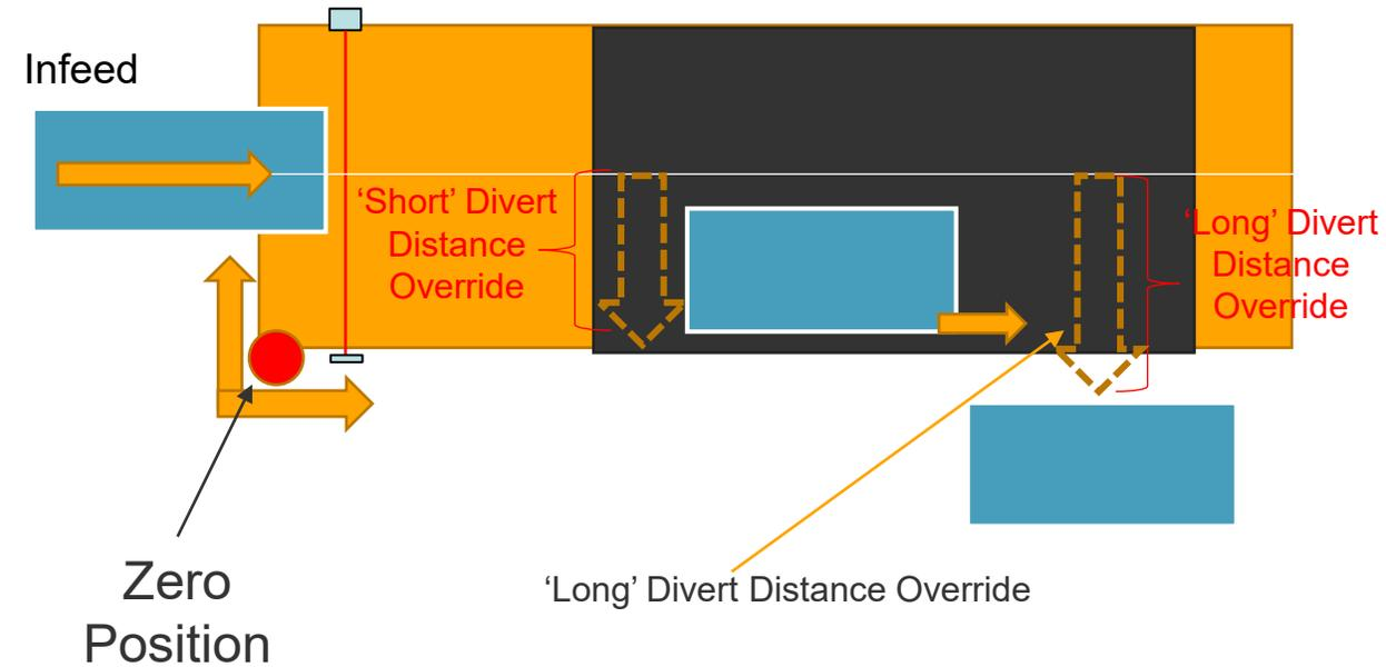
Trailing Edge: activation is triggered when trailing edge of the product reaches the start of activation area.
