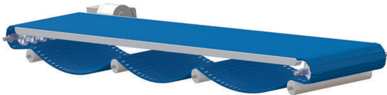
Figure 145: Full catenary returnway
