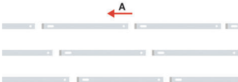
Figure 137: Straight, parallel wearstrip pattern
