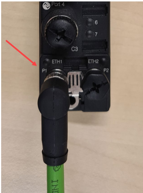
Figure 2: Network cable connection
