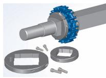
Figure 50: Heavy-duty split retainer ring
