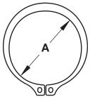
A Ring groove diameter Figure 52: Retainer ring groove diameter
