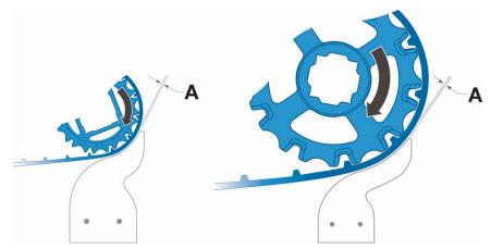
A 0.005–0.05 in (0.13–1.25 mm) spacing Figure 13: Correct limiter placement
