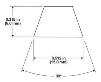
Figure 45: V-guide nominal geometry
