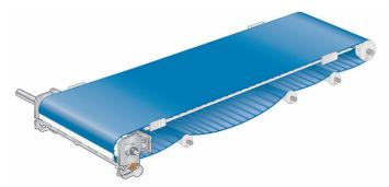
Figure 30: Catenary sag between components
