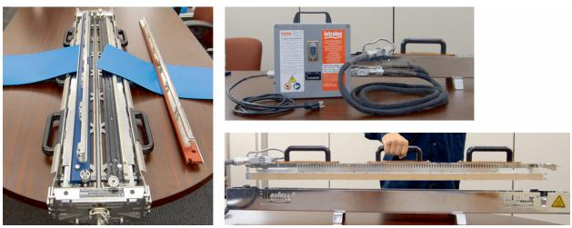
Figure 56: ThermoDrive Splicing System V2 and components
