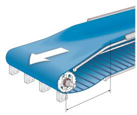
Ensure the transition distance (distance from end of troughed conveyor to drive or idle shaft center) is adequate. The transition distance must be a minimum of 1.5 times the belt width. Proper transition distance minimizes strain on belt edges and reduces belt friction.
