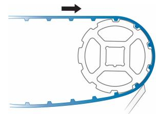
Figure 20: Scraper mounted at an angle
