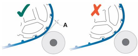
A 0.02 in (0.5 mm) spacing Figure 14: Correct placement of sprocket tooth beneath belt when setting the roller limiter
