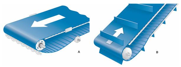
A Flat conveyor belt accumulation B Incline conveyor belt accumulation Figure 29: Belt accumulation
