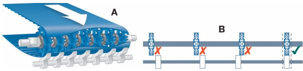
Figure 15: Correct alignment and minimum clearance for belts without accessories
