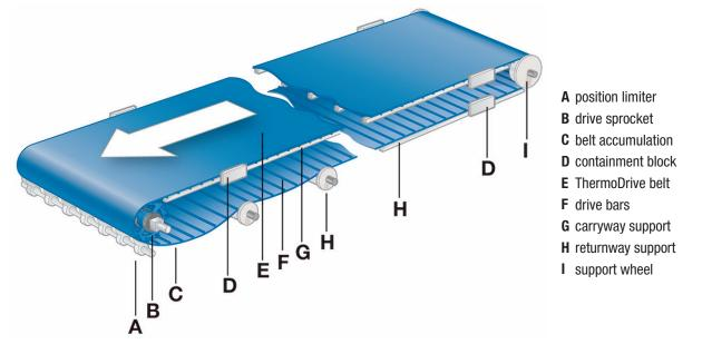
Figure 4: Conveyor belt components
