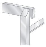
Figure 6: Correct joint assembly
