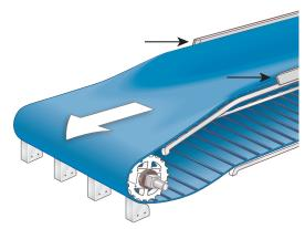
Use UHMW-PE containment rails or blocks for lateral belt containment. See Belt Containment.
