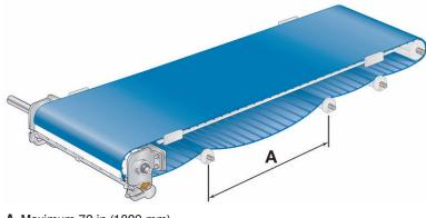
A Maximum 72 in (1829 mm) Figure 33: Correct support spacing
