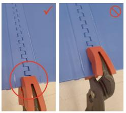
Figure 5: Clamp soft-jaw pliers on captive link
