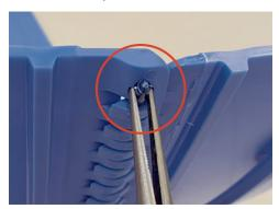
Figure 11: Use pliers to clamp rod
