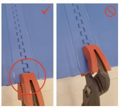
Figure 8: Clamp soft-jaw pliers on captive link
