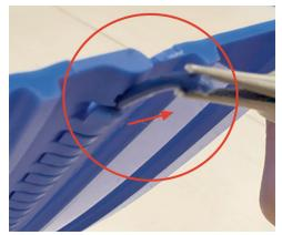
Figure 14: Pull rod out and away from belt
