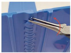
Figure 12: Twist pliers counterclockwise while maintaining pressure
