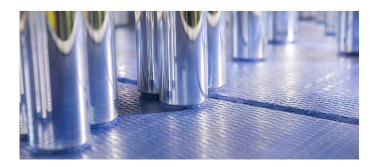
Intralox® Series 560 belting offers an exceptional tight transfer solution for mass can conveyance. Eliminating the need for dead plate transfers, S560 belting has been shown in field testing to reduce spoilage of 12-oz sleek cans by 70% compared to transfers with dead plates. S560 belting also prevents cans from becoming stranded on dead plates, reducing the risk of palletizing mixed labels and eliminating labor needed to clear the line of stranded cans at each label change.
