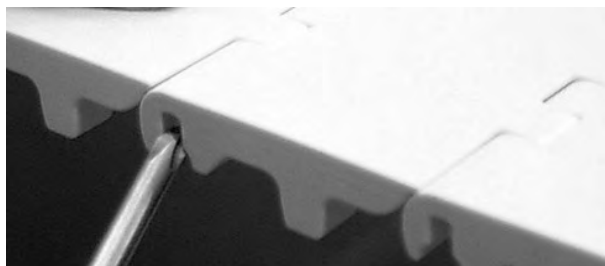
Figure 201: Push rod past retention figure
