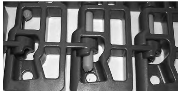
Figure 121: Ensure rod is fully inserted
