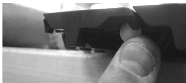
Figure 65: Push rod past retention feature
