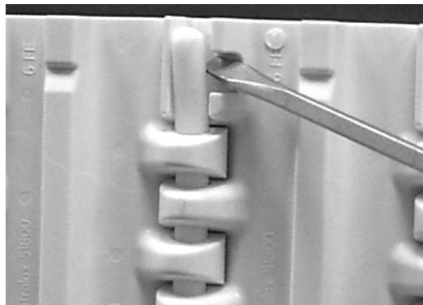
Figure 203: Lift rod over retention feature
