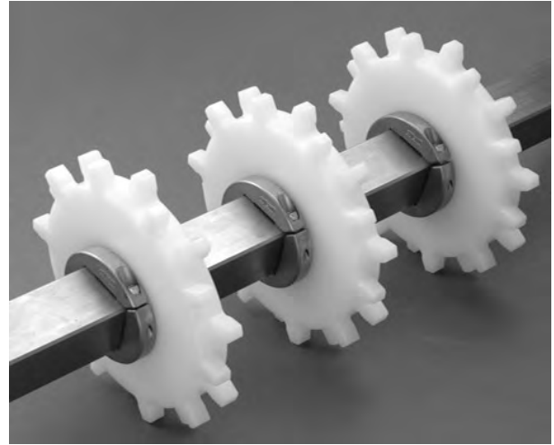
Figure 325: Secure both sides of all sprockets
