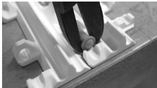
Figure 179: Cut rod head
