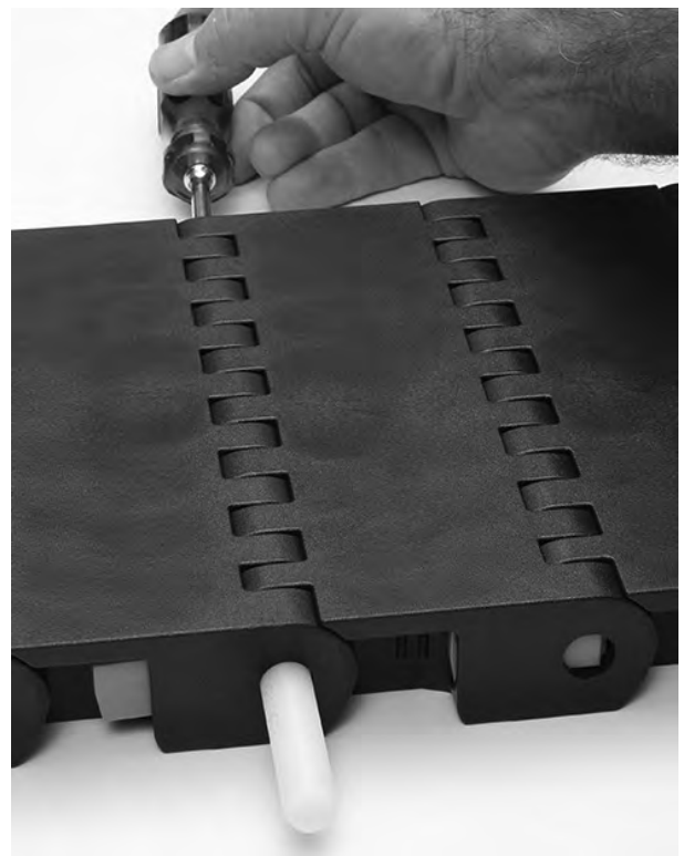
Figure 253: Push rod from belt
