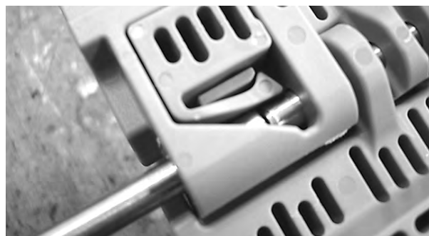
Figure 100: Push rod past retention feature
