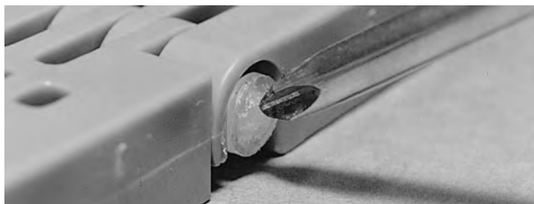
Figure 39: Ensure rod head is past snap-lock
