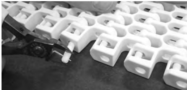
Figure 281: Pull rod from belt
