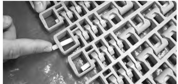
Figure 328: Push rod past retention feature
