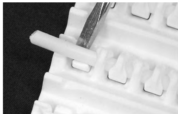
Figure 173: Lift rod over retention feature
