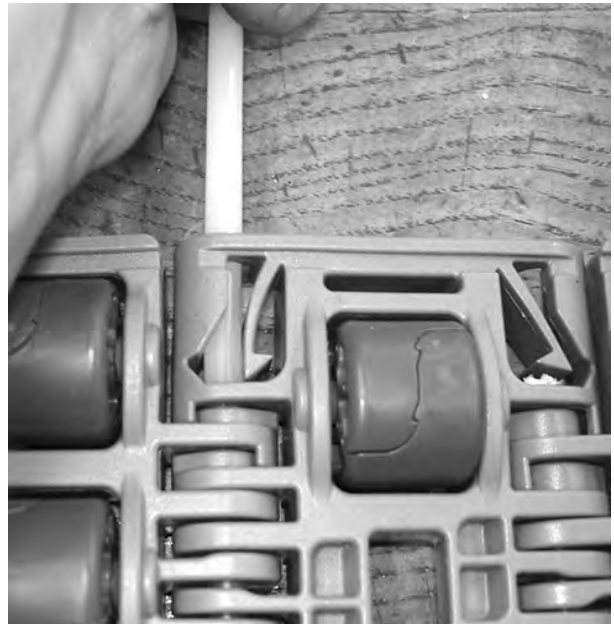
Figure 211: Push rod from belt
