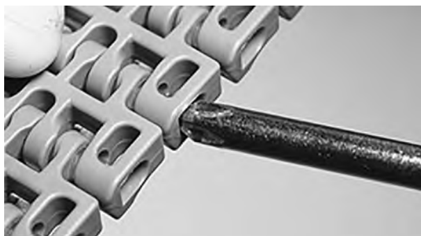
Figure 142: Push rod past retention feature
