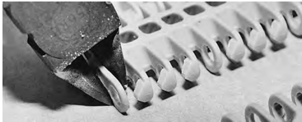
Figure 27: Cut outermost link
