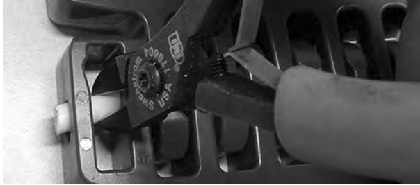
Figure 323: Push rod to side and past occluded hole
