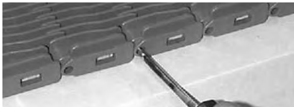
Figure 45: Push rod from belt
