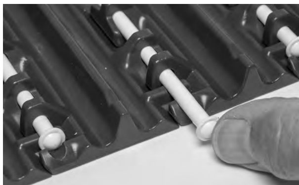
Figure 92: Insert rod through hinges
