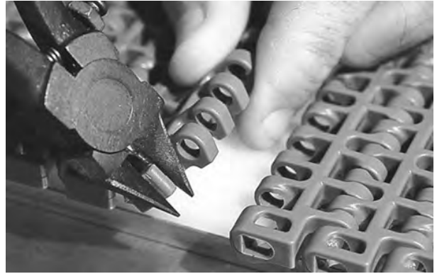
Figure 139: Cut edge from belt
