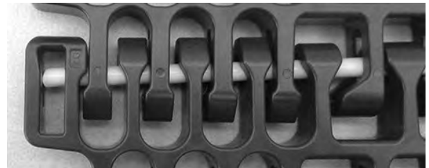
Figure 305: Ensure rod is past retention feature
