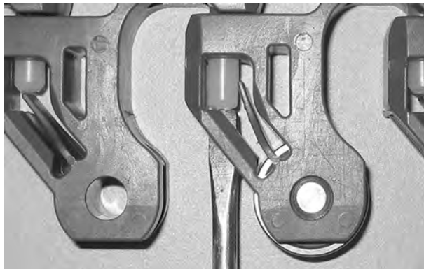
Figure 268: Push rod past retention feature
