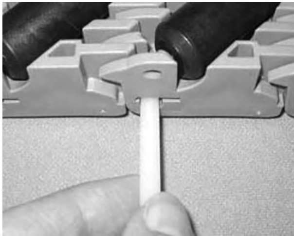
Figure 214: Insert rod through hinges
