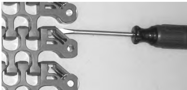
Figure 288: Open retention feature
