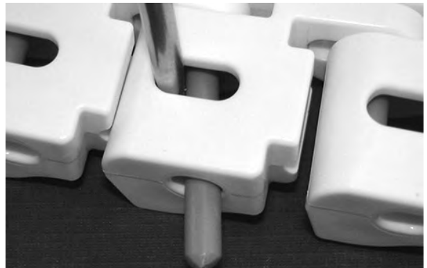
Figure 275: Push rod through retention feature
