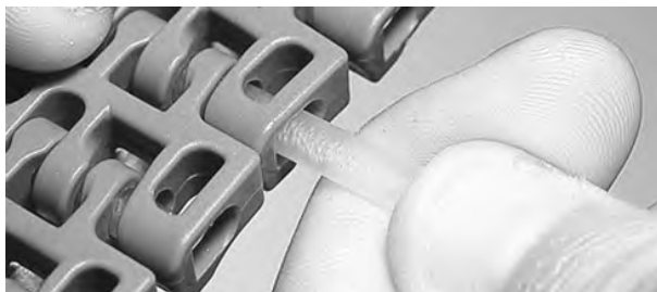
Figure 132: Insert rod through hinges
