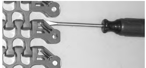
Figure 270: Open retention feature
