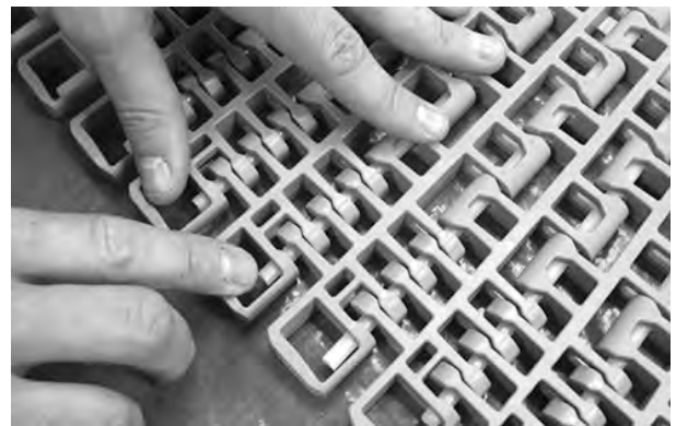
Figure 329: Ensure rod is past retention feature
