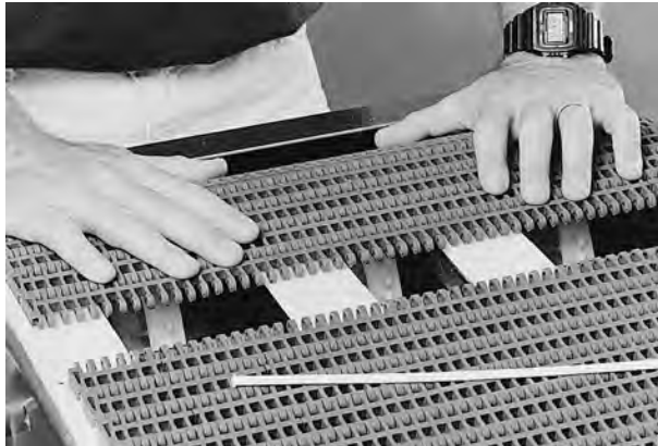
Figure 14: Push belt ends together
