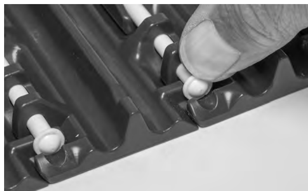
Figure 94: Push rod past retention feature
