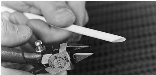
Figure 15: Clip rod at angle
