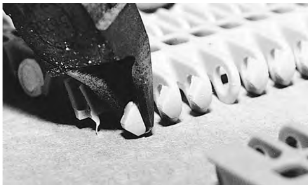
Figure 28: Cut spacer tip
