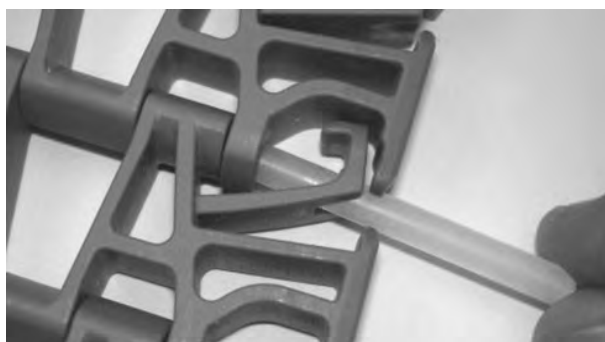
Figure 236: Insert rod through hinges
