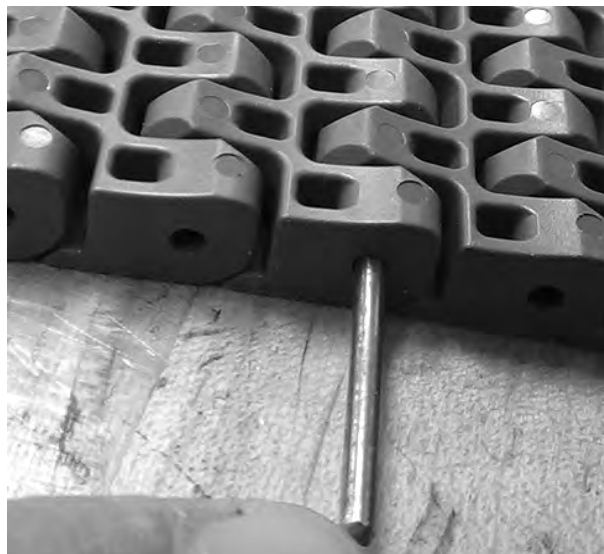
Figure 259: Push rod and rodlet from belt
