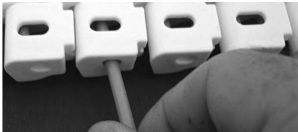
Figure 272: Insert rod through hinges
