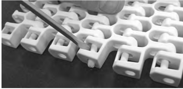
Figure 280: Push rod through retention feature
