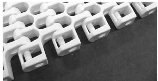
Figure 279: Ensure rod is past retention feature
