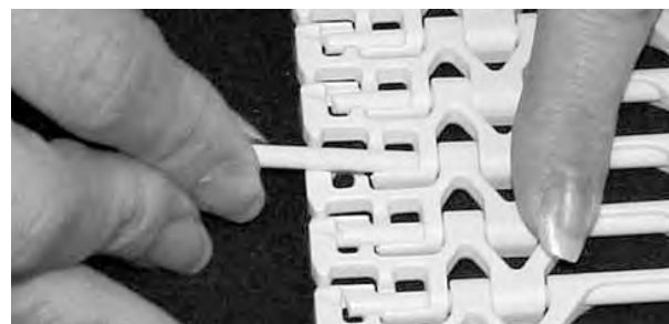
Figure 166: Insert rod through hinges
