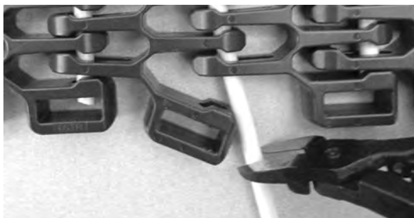
Figure 319: Pull rod from belt
