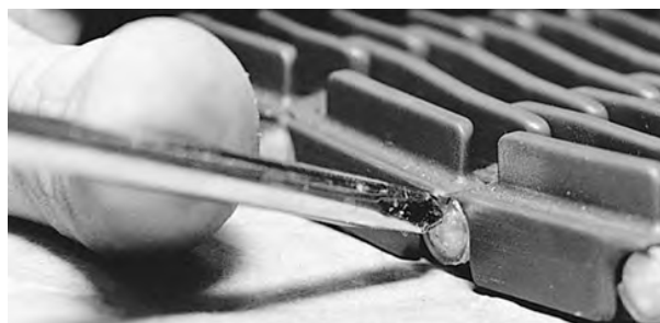
Figure 108: Ensure rod is past snap-lock
