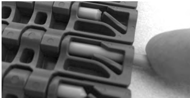
Figure 124: Insert rod through hinge
