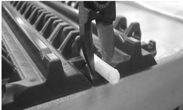
Figure 68: Pull rod from belt
