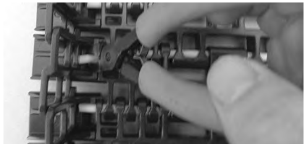
Figure 357: Push rod past retention feature
