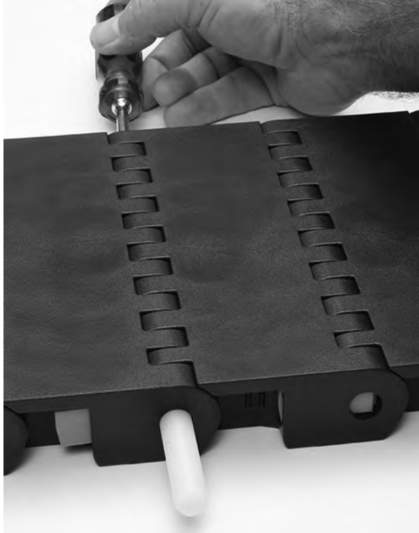
Figure 249: Push rod from belt
