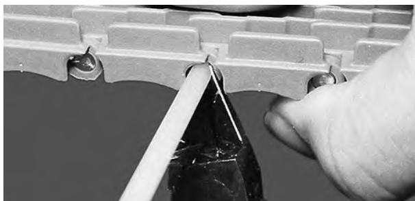
Figure 25: Cut rod flush with belt edge
