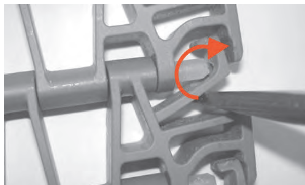
Figure 239: Rotate screwdriver to hold retention feature open
