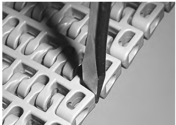
Figure 135: Push rod past retention feature
