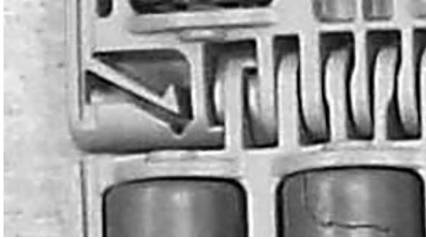
Figure 213: Ensure rod is past retention feature
