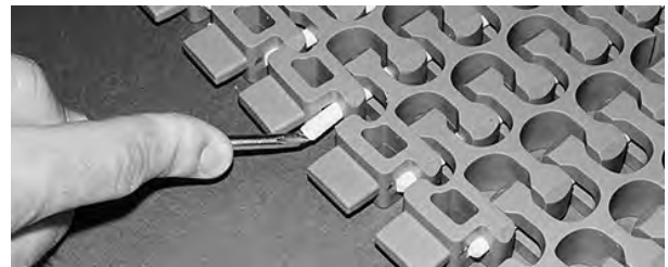
Figure 261: Ensure rod is past retention feature
