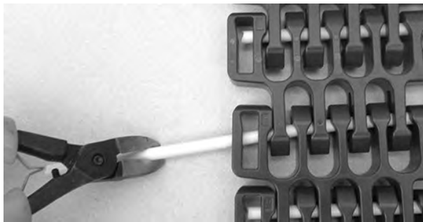
Figure 307: Pull rod from belt
