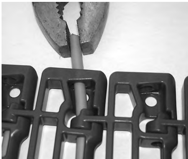
Figure 123: Pull rod from belt
