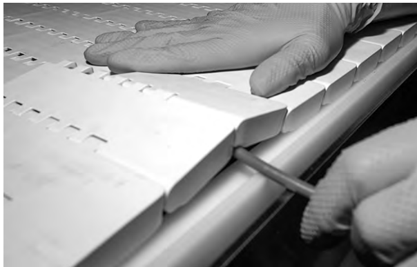
Figure 84: Slightly bend and insert rod through hinges
