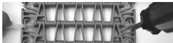
Figure 240: Push rod from belt
