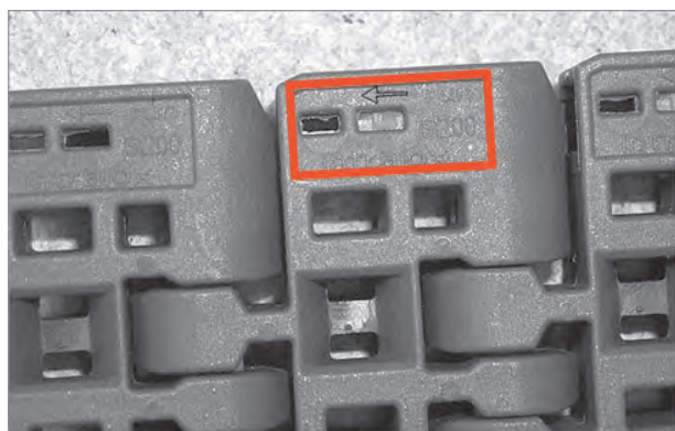
Figure 151: Belt running direction
