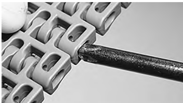
Figure 133: Push rod past retention feature
