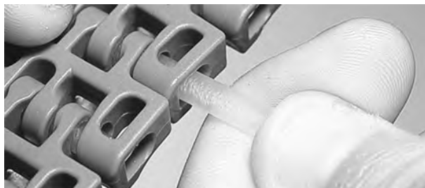
Figure 141: Insert rod through hinges
