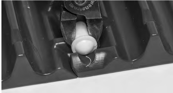
Figure 96: Cut rod head
