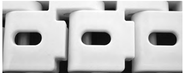
Figure 274: Ensure rod is past retention feature
