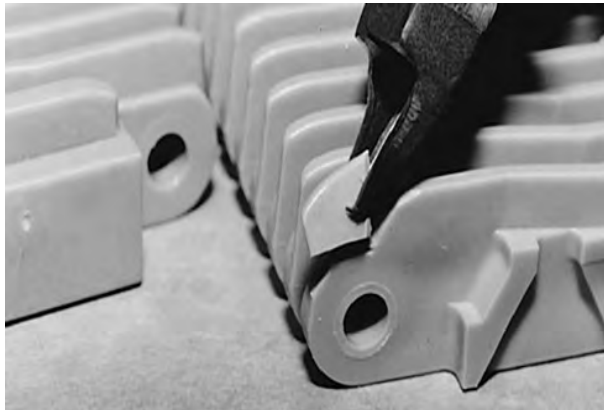
Figure 48: Cut outermost rib
