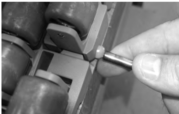
Figure 187: Push rod past retention feature
