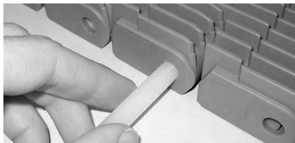
Figure 208: Pull rod from belt
