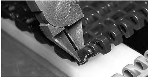
Figure 137: Cut off half of edge
