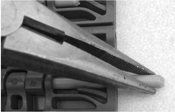
Figure 128: Pull rod from belt
