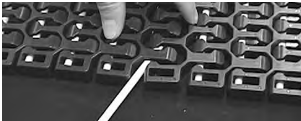
Figure 294: Insert rod through hinges
