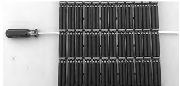
Figure 233: Push rod from belt
