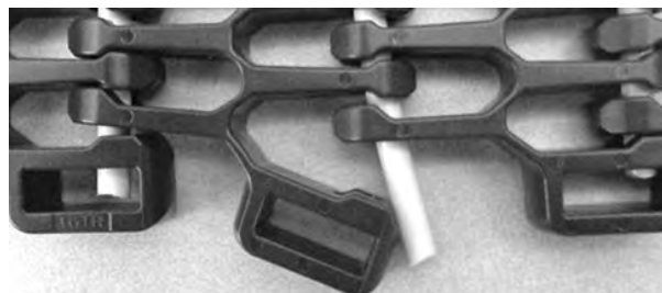
Figure 315: Push rod past belt edge
