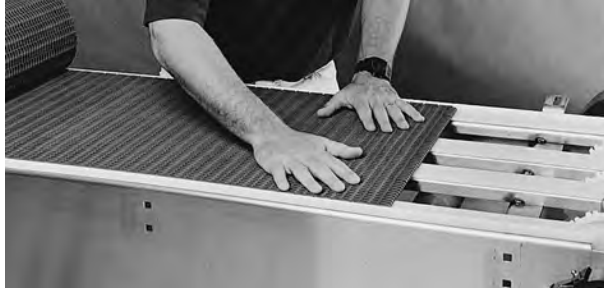
Figure 9: Feed belt from drive end
