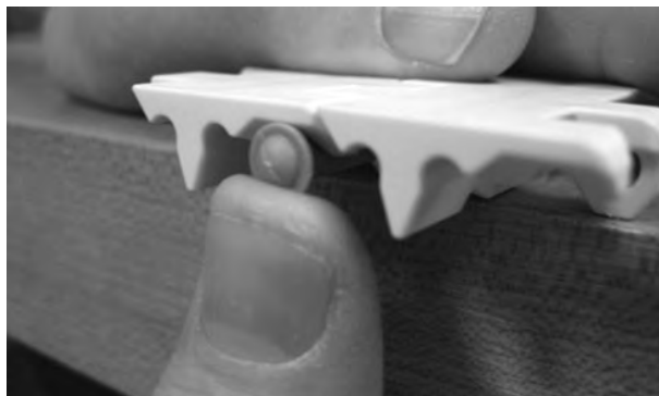
Figure 176: Use thumb to push rod
