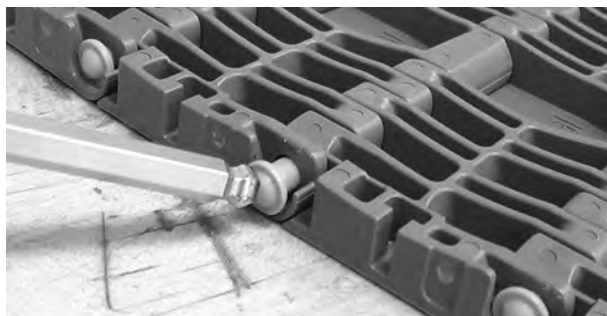
Figure 257: Push rodlet past retention feature
