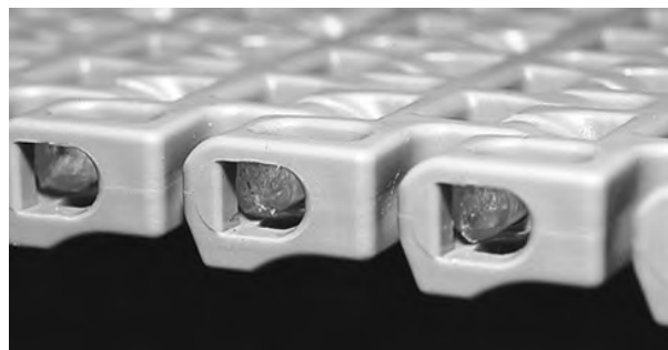
Figure 143: Ensure rod is past retention feature
