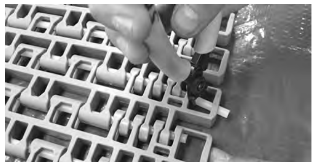
Figure 330: Pull rod from belt
