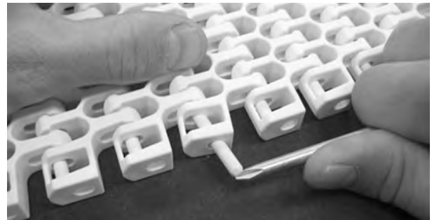
Figure 278: Push rod past retention feature
