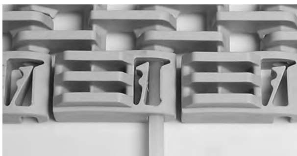
Figure 80: Push rod into belt
