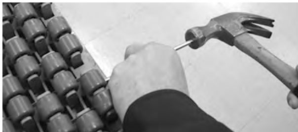
Figure 191: Push rod from belt
