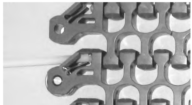
Figure 271: Push rod from belt
