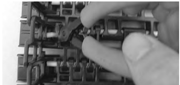
Figure 343: Pull rod from belt
