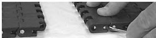
Figure 157: Use screwdriver to close Slidelox
