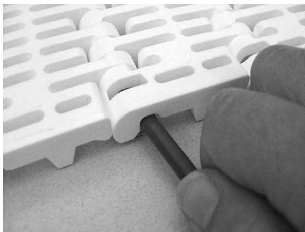
Figure 75: Push rod into belt
