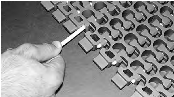
Figure 265: Pull out rod
