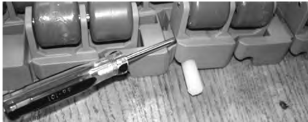
Figure 192: Pull rod from belt
