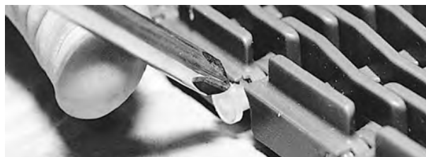
Figure 107: Push rod into belt
