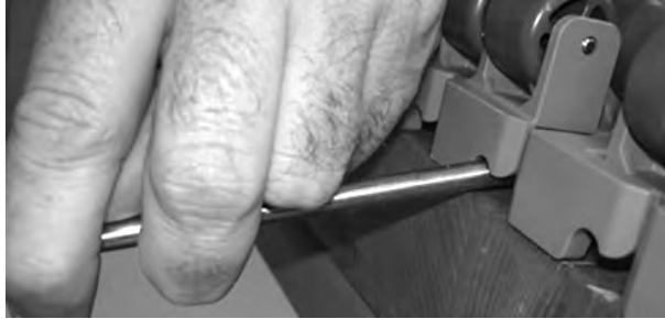
Figure 190: Insert steel pin in hinge
