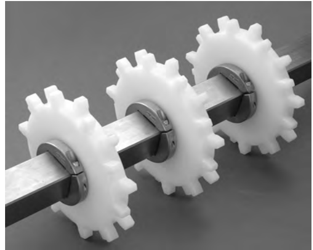
Figure 308: Secure both sides of all sprockets
