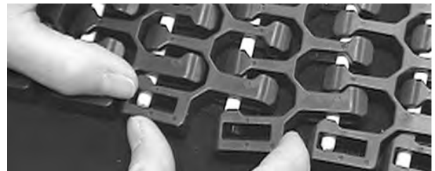
Figure 297: Push rod past belt edge, snap flush edge over rod
