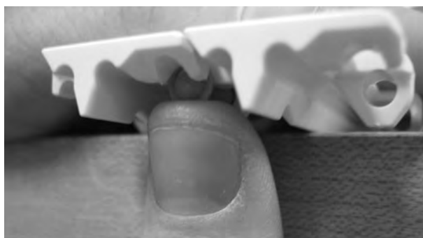
Figure 177: Push rod past retention feature
