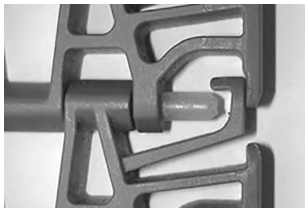
Figure 238: Ensure rod is past retention feature
