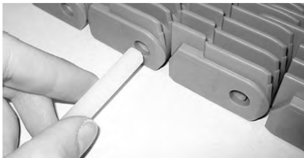
Figure 205: Insert rod through hinges
