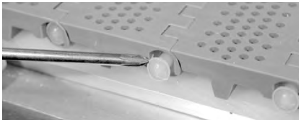
Figure 59: Push rod into belt
