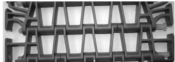
Figure 245: Ensure rod is past retention feature
