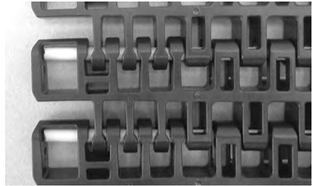
Figure 346: Ensure rod is past retention feature
