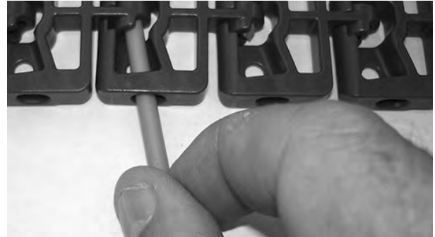
Figure 119: Insert rod through hinges
