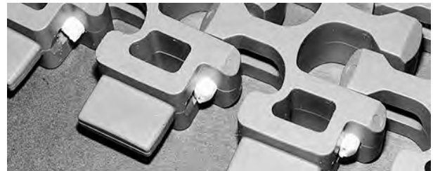
Figure 262: Ensure rod is fully inserted
