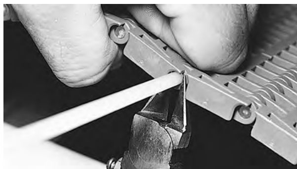
Figure 109: Cut rod flush with belt edge
