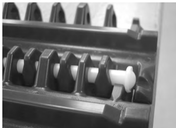
Figure 66: Ensure rod is past retention feature
