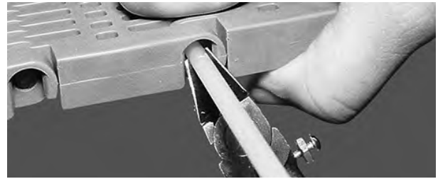
Figure 40: Cut rod flush with belt edge
