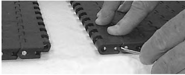
Figure 159: Close the Slidelox
