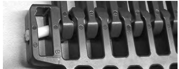
Figure 321: Insert rod through hinges
