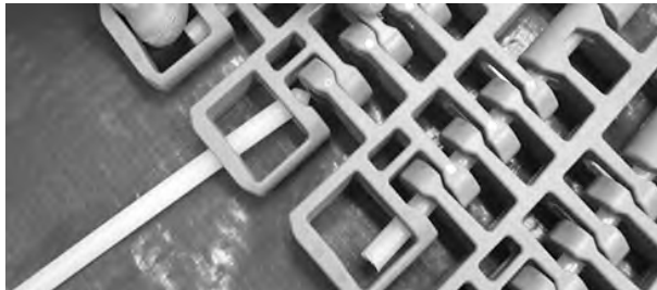
Figure 327: Insert rod through hinges
