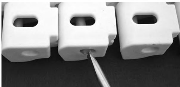
Figure 273: Push rod past retention feature
