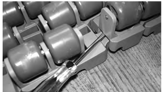
Figure 189: Insert screwdriver under roller
