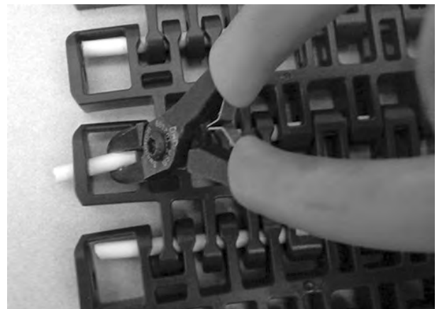
Figure 347: Push rod past retention feature
