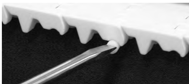
Figure 171: Push rod past retention feature
