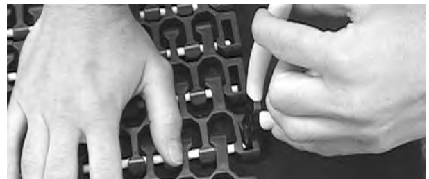
Figure 299: Push rod into belt
