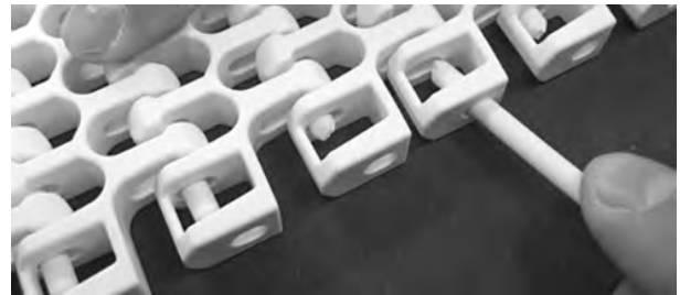
Figure 277: Insert rod through hinges
