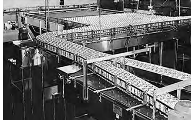
Figure 18: Place supports across width of belt
