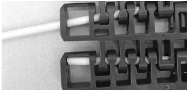
Figure 344: Insert rod through hinges
