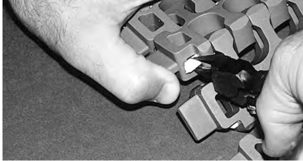
Figure 263: Free rod from retention feature
