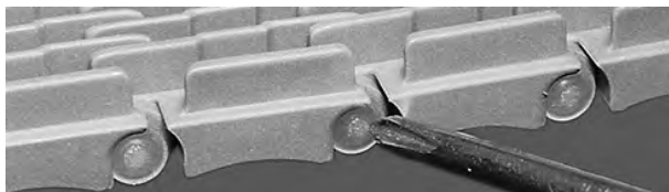
Figure 24: Ensure rod head is past snap-lock
