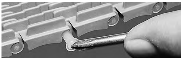
Figure 23: Push rod into belt
