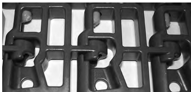
Figure 112: Rods move inside flush edge
