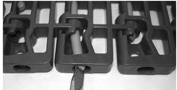
Figure 120: Push rod past retention feature
