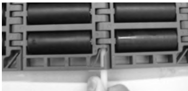
Figure 226: Insert rod through hinges
