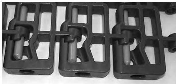
Figure 113: Rod grows into flush edge
