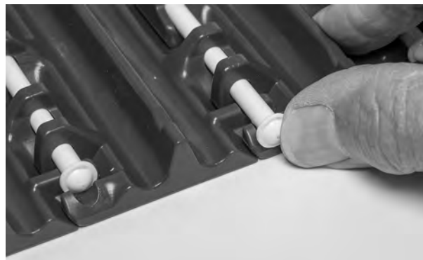
Figure 93: Use thumb to push rod
