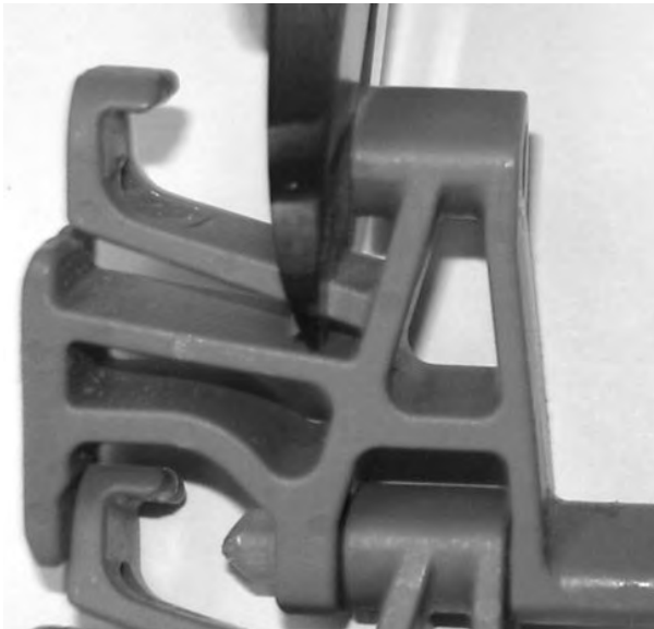
Figure 242: Cut retention feature
