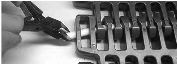
Figure 324: Pull rod from belt
