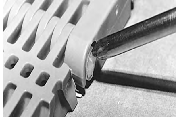
Figure 49: Push rod head past retention feature
