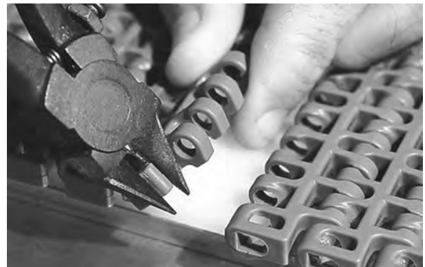
Figure 149: Cut edge from belt
