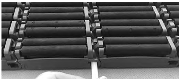
Figure 230: Insert rod through hinges
