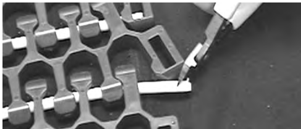
Figure 302: Pull rod from belt
