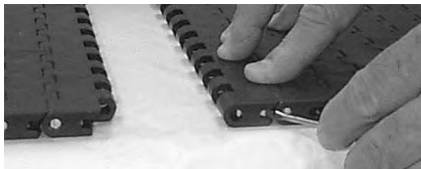
Figure 163: Close the Slidelox
