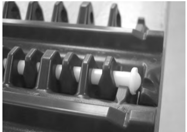
Figure 71: Ensure rod is past retention feature
