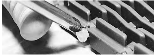
Figure 107: Push rod into belt
