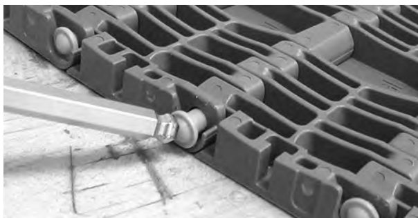
Figure 272: Push rodlet past retention feature
