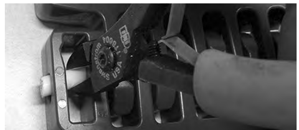
Figure 338: Push rod to side and past occluded hole
