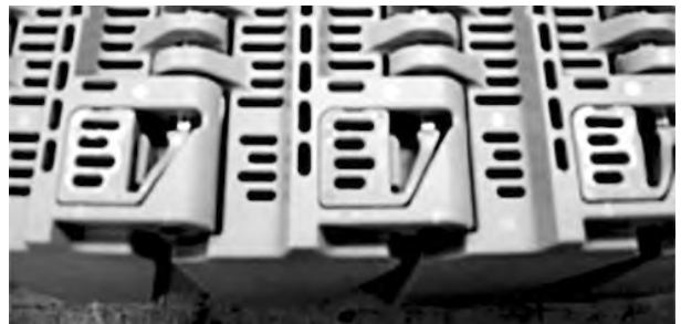
Figure 101: Ensure retention feature is closed
