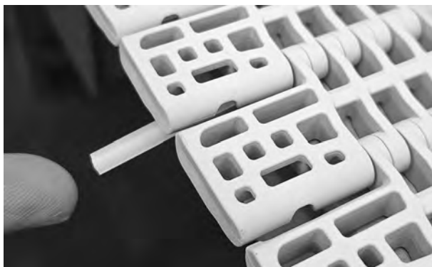
Figure 125: Push rod until it snaps into flush edge
