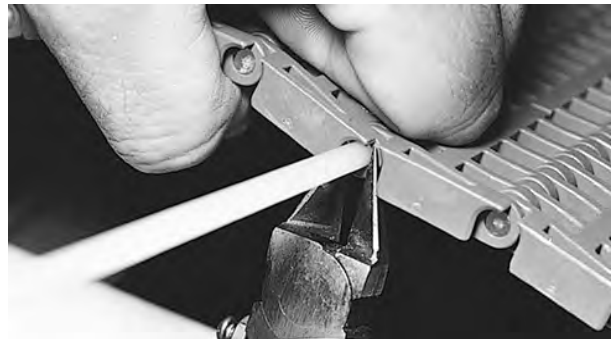
Figure 109: Cut rod flush with belt edge
