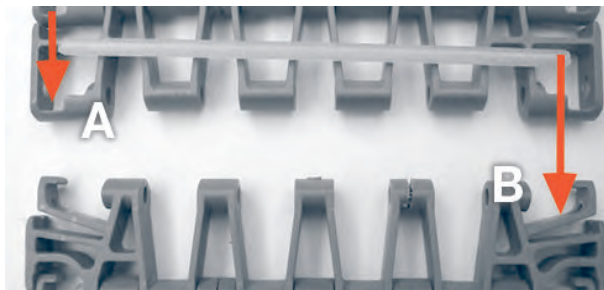
A Original belt section B New belt section
