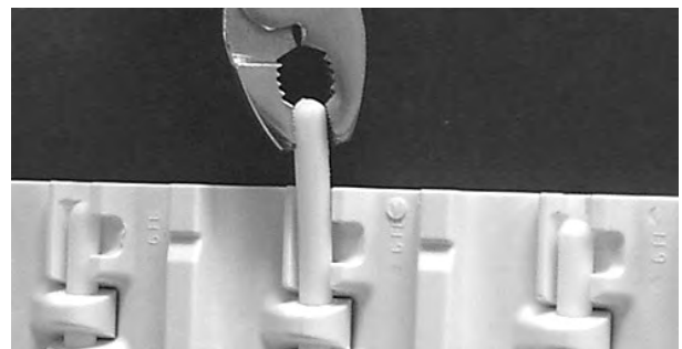
Figure 208: Pull rod from belt
