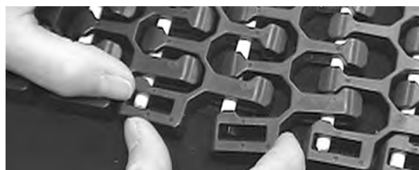
Figure 312: Push rod past belt edge, snap flush edge over rod
