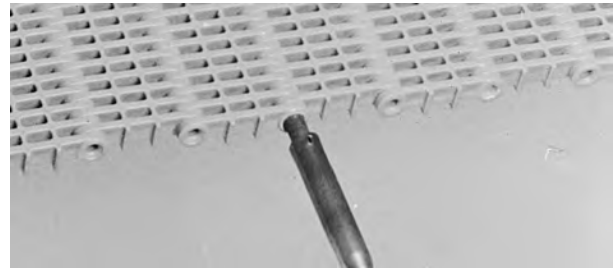
Figure 36: Close rod hole
