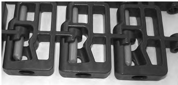
Figure 113: Rod grows into flush edge
