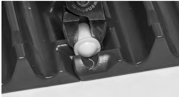
Figure 96: Cut rod head
