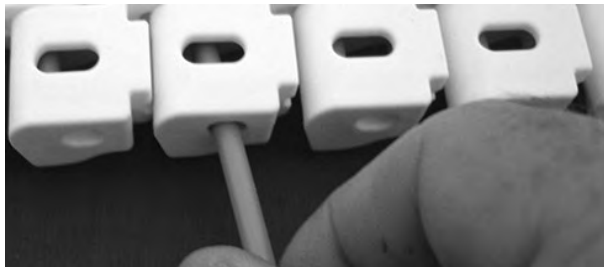
Figure 287: Insert rod through hinges
