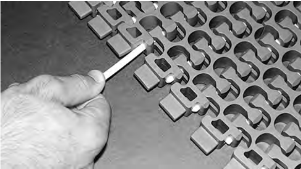
Figure 280: Pull out rod
