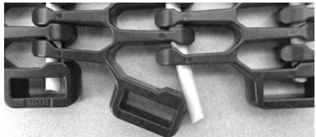
Figure 330: Push rod past belt edge
