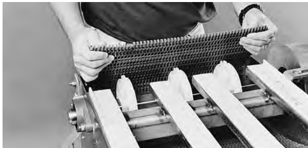
Figure 17: Feed belt down returnway
