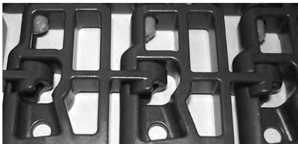
Figure 112: Rods move inside flush edge
