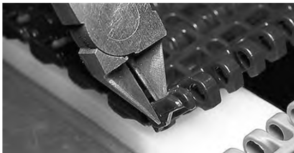
Figure 151: Cut edge member
