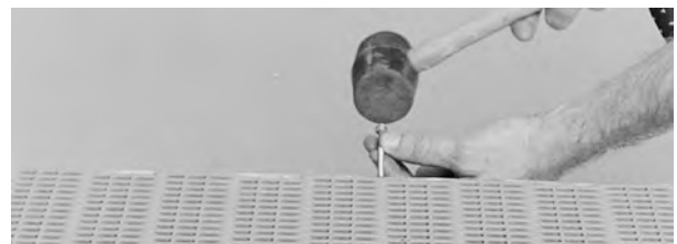
Figure 38: Push rod from belt
