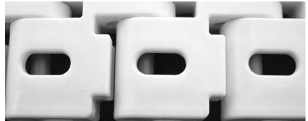
Figure 289: Ensure rod is past retention feature
