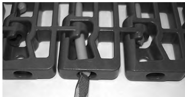
Figure 120: Push rod past retention feature
