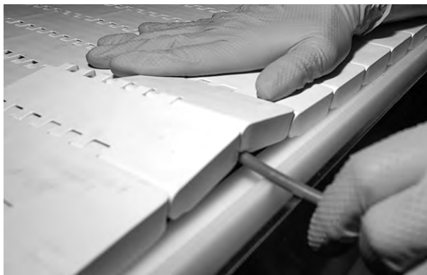
Figure 89: Slightly bend and insert rod through hinges
