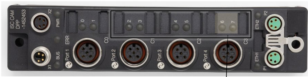
LED 6-7: Used for 24v reject connection Figure 6: C3 connect of 24v reject signal
