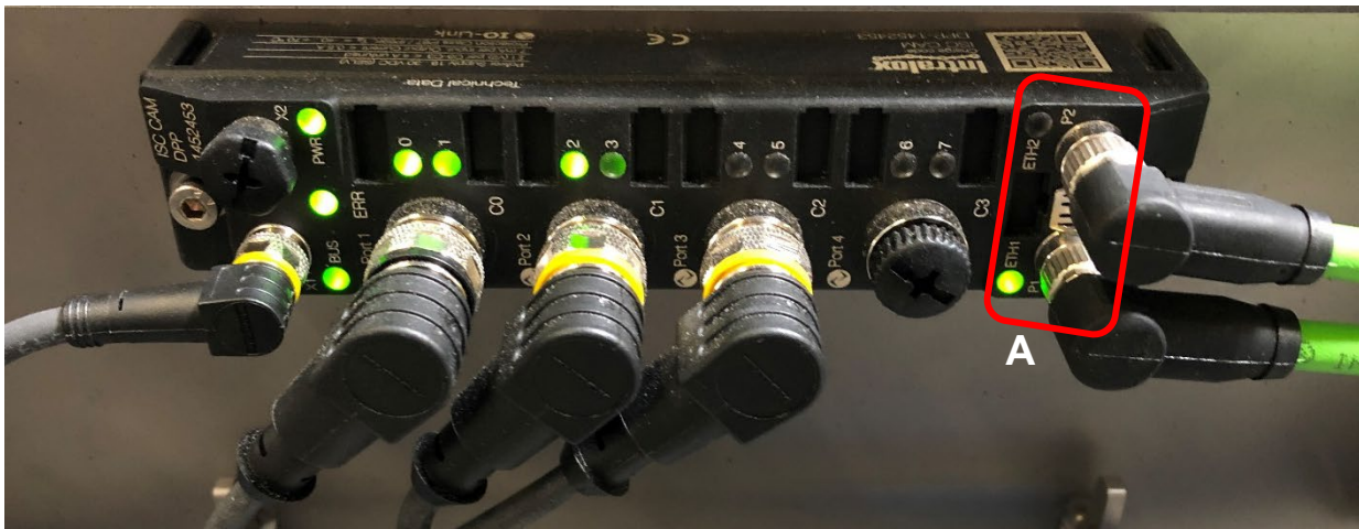
A Ethernet: ETH1 and ETH2 LED indicators
