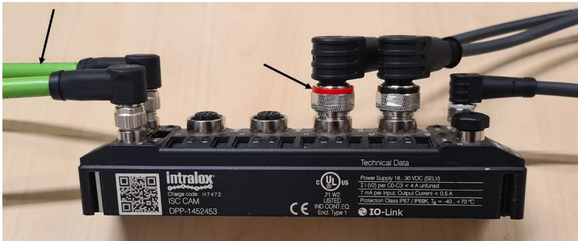
Figure 7: Cable connections and color coding
