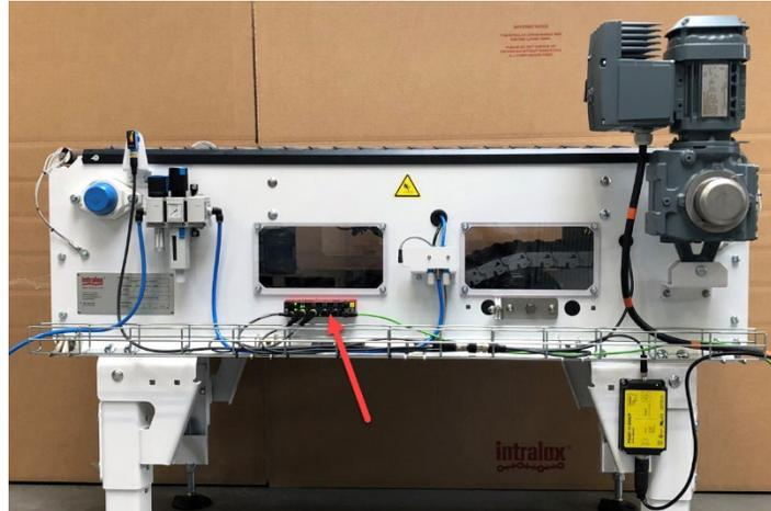
Figure 6: Install ISC CAM to side panel
