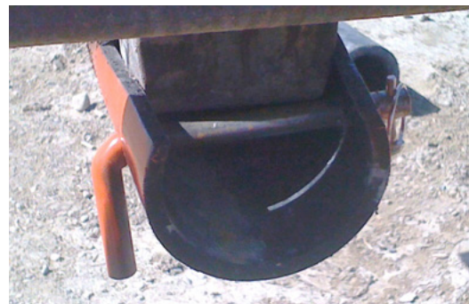
Figure 7: Fork pad securing
