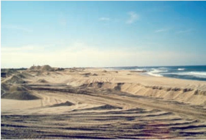
FIG 1.3 Beach-sand mining in Portugal. In this case, the sand is being mined from a very wide beach created by a large jetty or rock wall perpendicular to the beach that traps sand on its updrift or upstream side, much like a river dam. Just like a dam, the downdrift or downstream beach side (not shown here) is missing a lot of sand, and that shoreline is rapidly eroding. If the beach were to need nourishment, sand could be removed from upstream and placed on the downdrift side of the jetty, or sand could be brought in from inland sources. Photo by William Neal.
