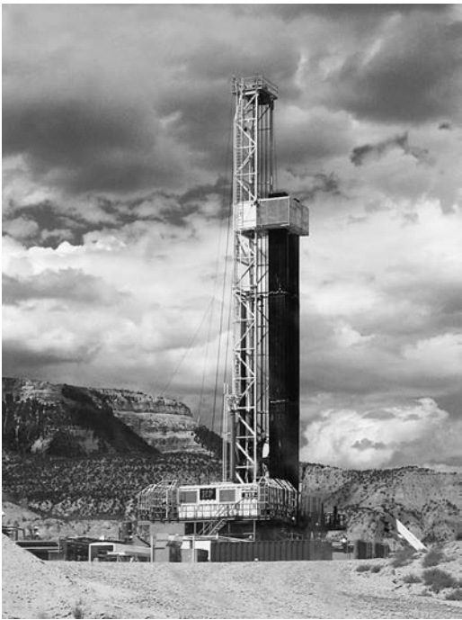
FIGURE 1.5. Flex rig for directional drilling. Photo by the author.
