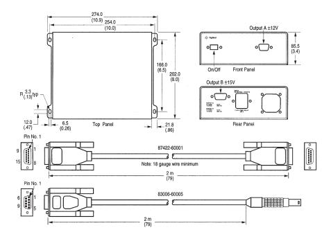
The Keysight 87422A power supply provides the dc power needed to bias the 83020A. DC cables shown above shipped with power supply. Dimensions in millimeters and (inches).
