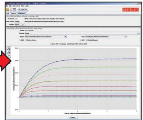
Performing nested sweeps to characterize a transistor with TSP Express is quick and easy. Data can be exported to a .csv file for use with spreadsheet applications such as Excel®.
