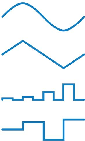
Current arbitrary waveforms maximum output update rates: 12,500 samples/second.
