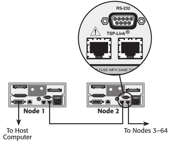
Each SourceMeter instrument has two TSP-Link connectors to facilitate chaining instruments together.
