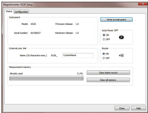
Status screen allows you to assign a unique name for the instrument and to check and clear memory as needed.
