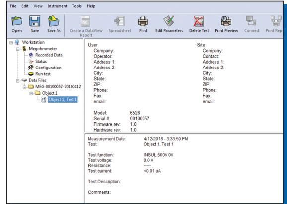
Tree structured status screen provides the ability to select connected instruments, configure instruments, see the instrument's status and review stored test results.
