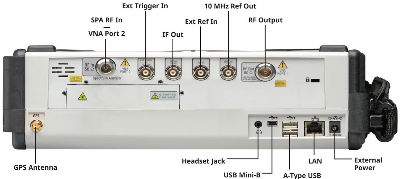
All connectors are conveniently located on the top panel, leaving the sides clear for handheld use
