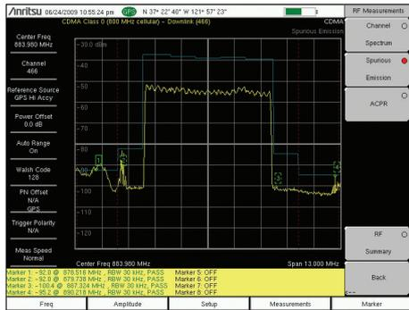
**RF Measurements – Spectral Emissions Mask**
