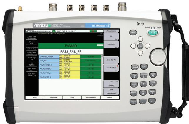
BTS Master in RF Measurements Pass/Fail Mode
