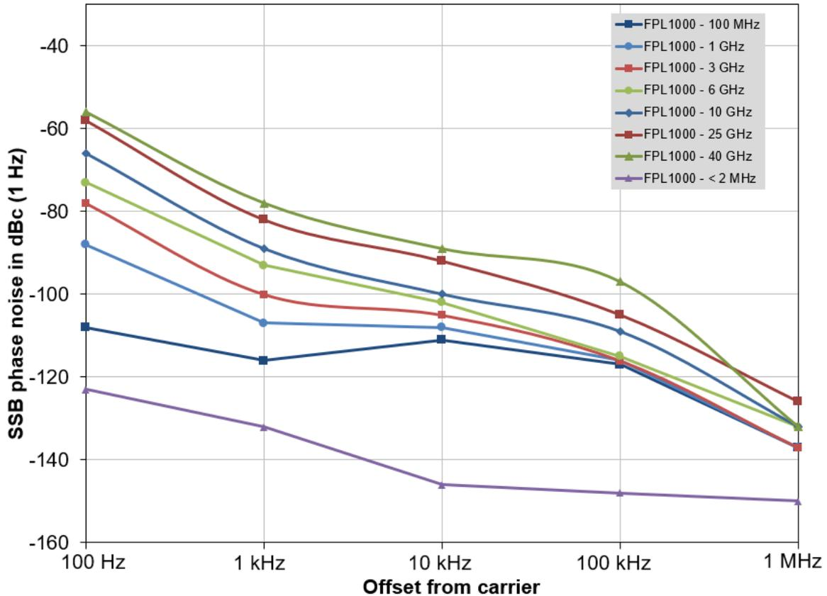
Measured SSB phase noise at different center frequencies
