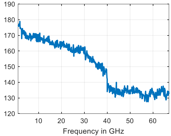
Exemplary measured dynamic range for R&S®ZNA43 (left) and R&S®ZNA67 (right) in reversed coupler configuration (-B16) at maximum output power, receiver step attenuator set to 0 dB at 1 Hz resolution bandwidth
